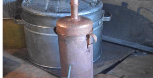
Boiler for țuica (a traditional Romanian spirit that contains ~ 24-65% alcohol by volume)
