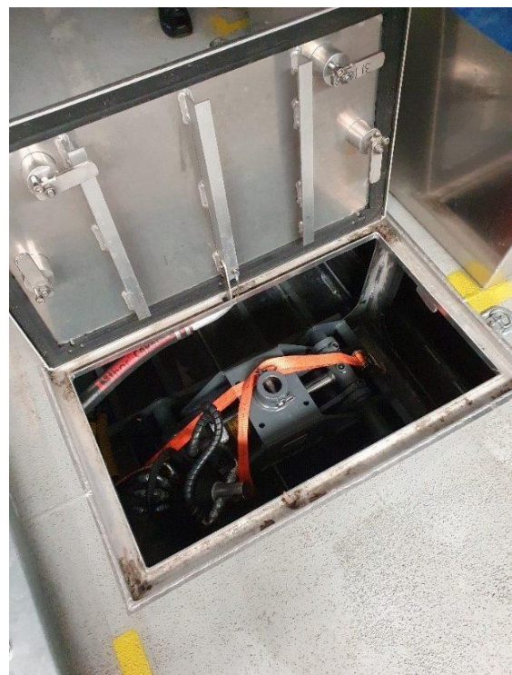
THE GRAB IS PLACED BELOW DECK, ALLOWING MORE SPACE ON THE SHIP WHEN NOT IN USE (PHOTO: KIA F. PETERSEN)
