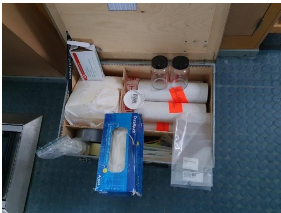
SAMPLING BOX WITH DIFFERENT EQUIPMENT TO ENSURE SAFE AND SECURE SAMPLING OF OIL AND OTHER SUBSTANCES AT SEA (PHOTO: KIA F. PETERSEN)
