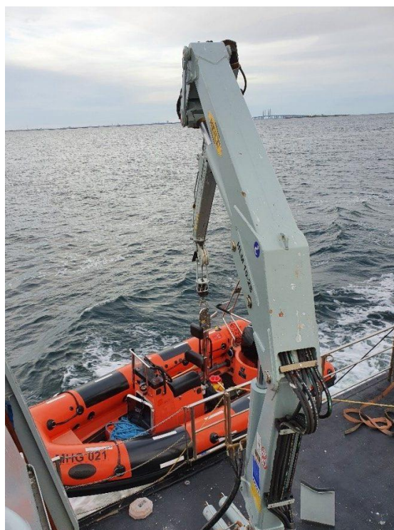
A RHIB IS LIFTED OFF THE SHIP BY CRANE (PHOTO: KIA F. PETERSEN)
