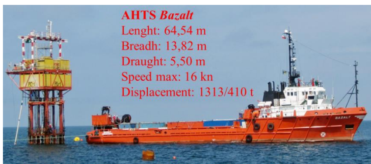
Fig. 2. AHTS 'Bazalt' with diving complex AF2 placed aft [http://www.tsmanagement.pl/flota (access 06.04.2017)]
