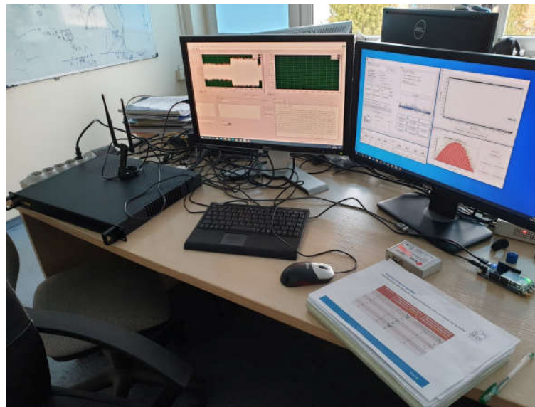
Figure 7-1: Integration of a sample recording module with a signal correlation module that determines pseudoranges a)
