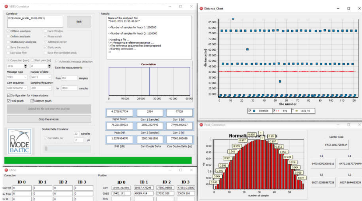
Figure 6-17: Signal correlation application - scenario for four stations
