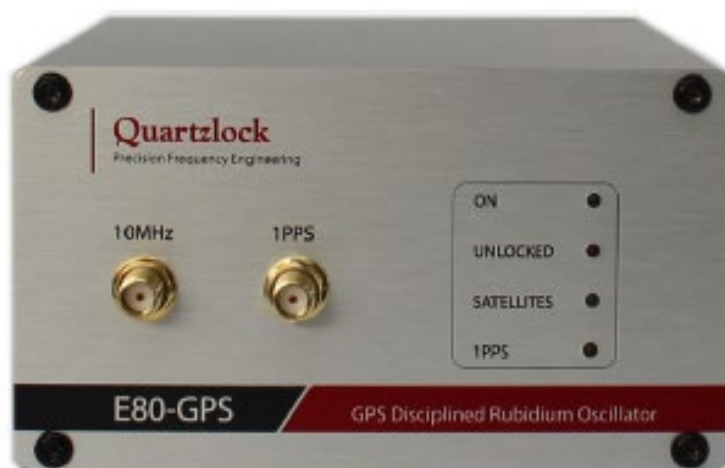
Fig. 3.1 The Quartzlock E80-GPS rubidium oscillator used at the R-Mode VDES station in the port of Gdynia
