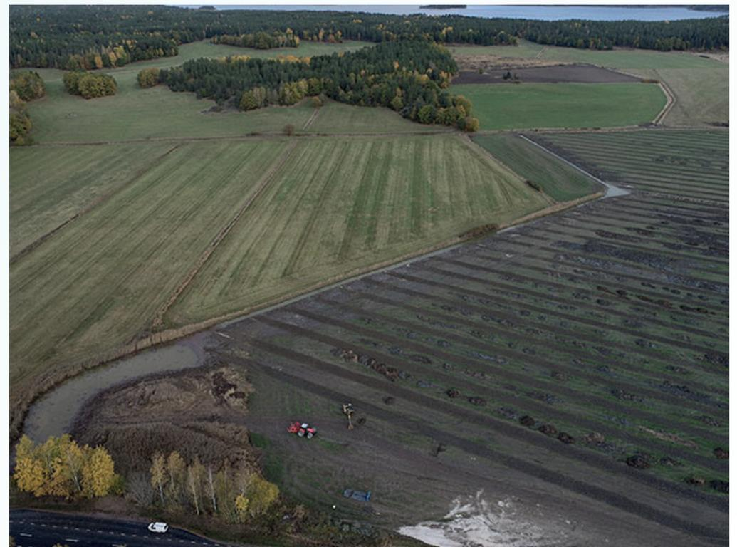
Structure liming, Filter ditches, and Phosphorus pond
