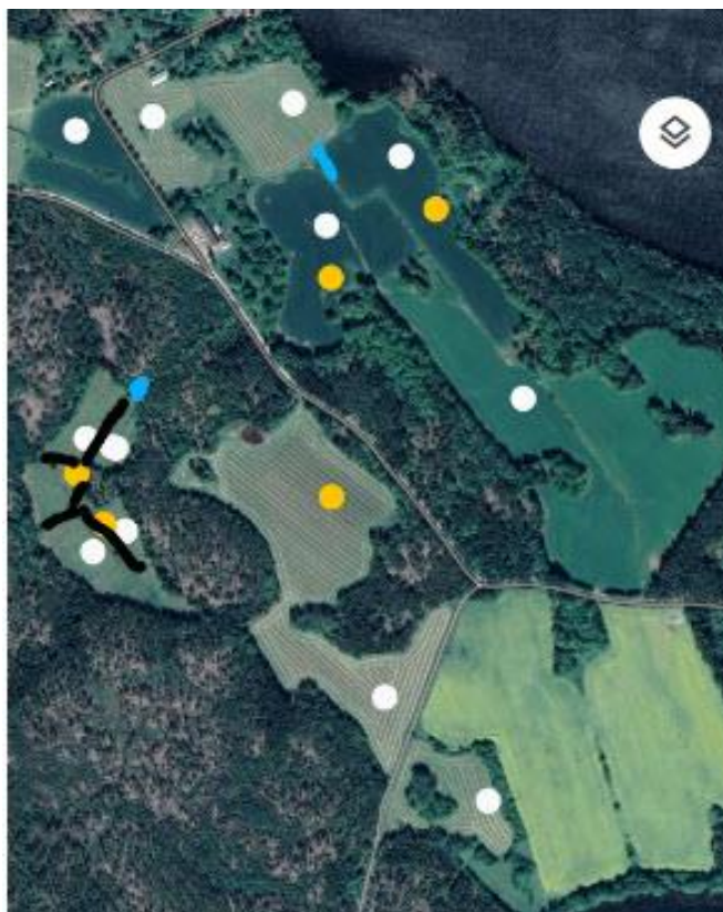
Local investment plan on farm level. White dots are planned structure liming, yellow dots – planned filter ditches, blue – small wetlands, black – two step ditches
