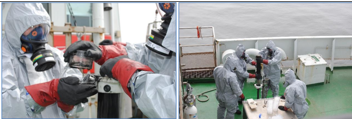
Fig. 1 & 2. Sediment sampling with protective clothes, gloves and breathing masks.
