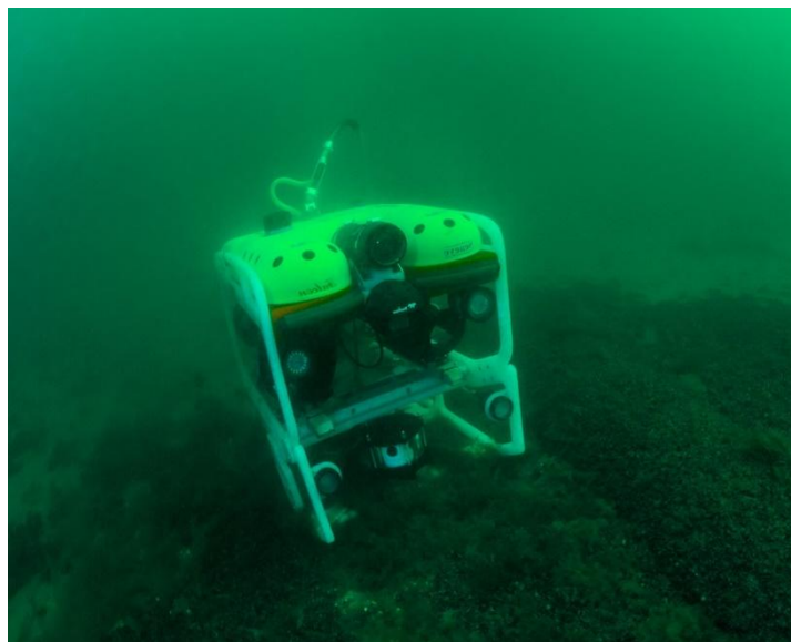
Fig. 3 Example ROV equipped with sediment sampler, video camera, lights, and the BlueView sonar
