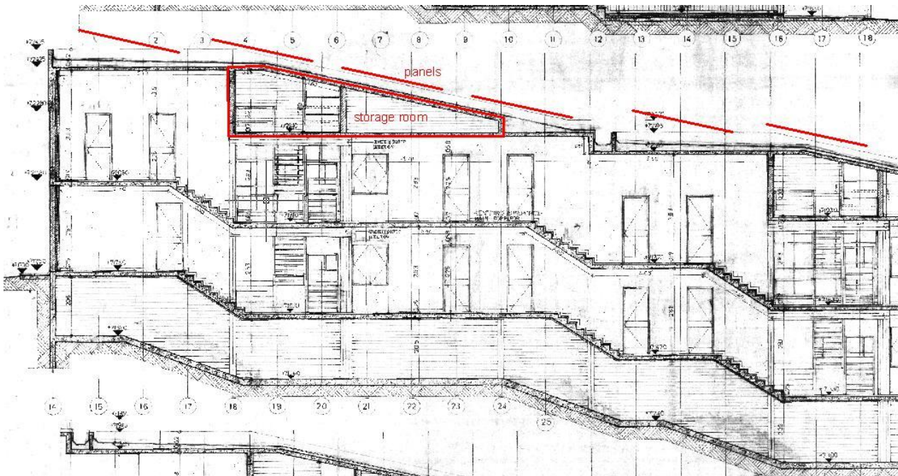
Figure 12: Section of the PV system in dormitories roof and storage room
