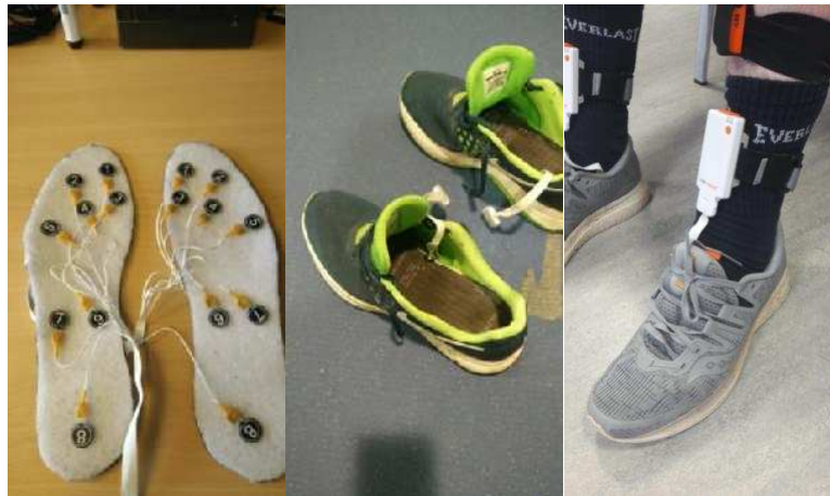
Figure 25: Walkinsense smart insole showing sensor layout, show insertion and leg attachment.
