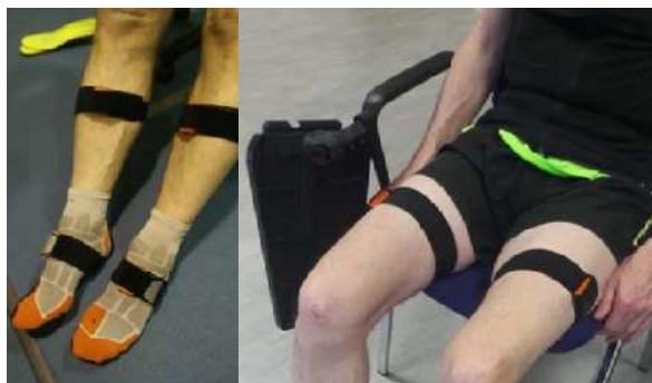
Figure 24: Xsens IMC system showing IMU positions for foot, lower leg and upper leg.
