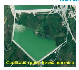
Summary: A mesocosm study and computer modelling were conducted to investigate if P fertilization of mine ponds can be used to increase N removal through denitrification. Denitrification did increase both in the mesocosm test and in a computer model of the Kiruna mine pond. The method needs further testing before fullscale implementation. Work was conducted in cooperation with Swedish University of Agricultural Sciences, Uppsala.
