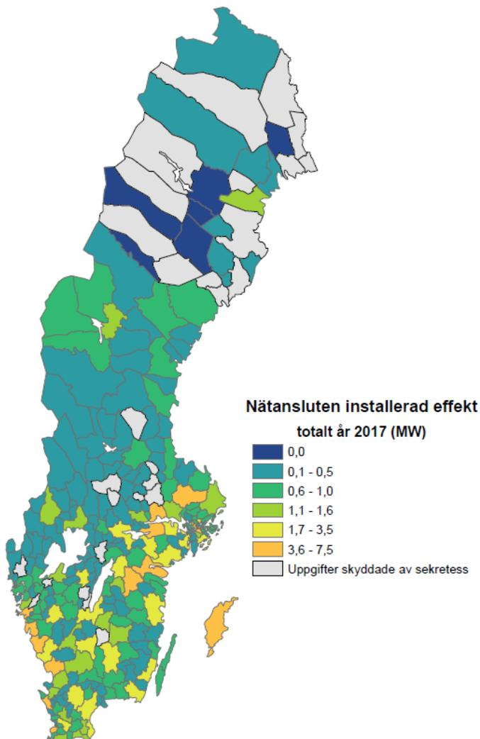
Sweden is lagging behind in PV development, in general, but even more in Northern Regions as the map shows. This is also due to the subsidy system: Sweden does not have a system of guaranteed feed in tariffs. Instead, income from PV plants comes from a variety of sources and is limited by a set of rules to some extent. More details below.
