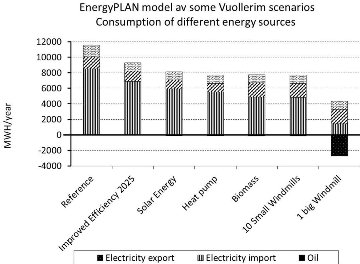
Wind power is only shown with up to 1 big windmill in this diagram. (Otherwise the scale would make it difficult to read the differences up to the installation of windmills). We see that the effect of the big windmill is a combination of less consumption from the net and export to the net.
