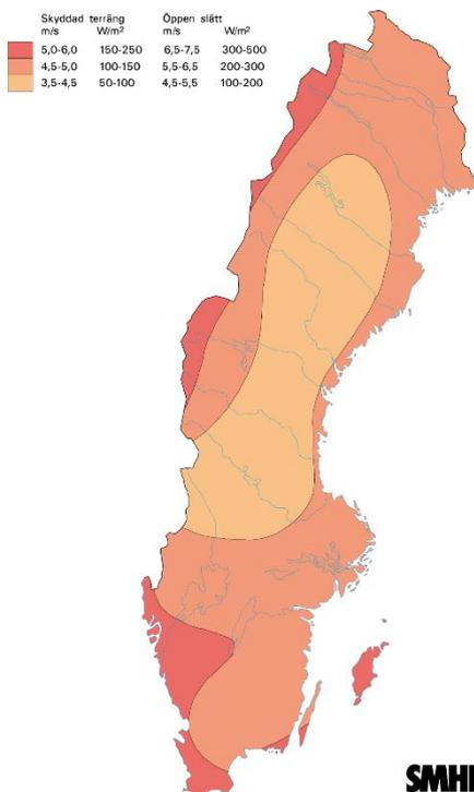
The wind energy with measurements in 50 m heights, Source SMHI, lies about 4.5 - 5,0 m/s and 100-150 W/m<sup>2</sup> in sheltered areas and 5.5-6,5 and 200-300 W/m<sup>2</sup> in more open areas.
