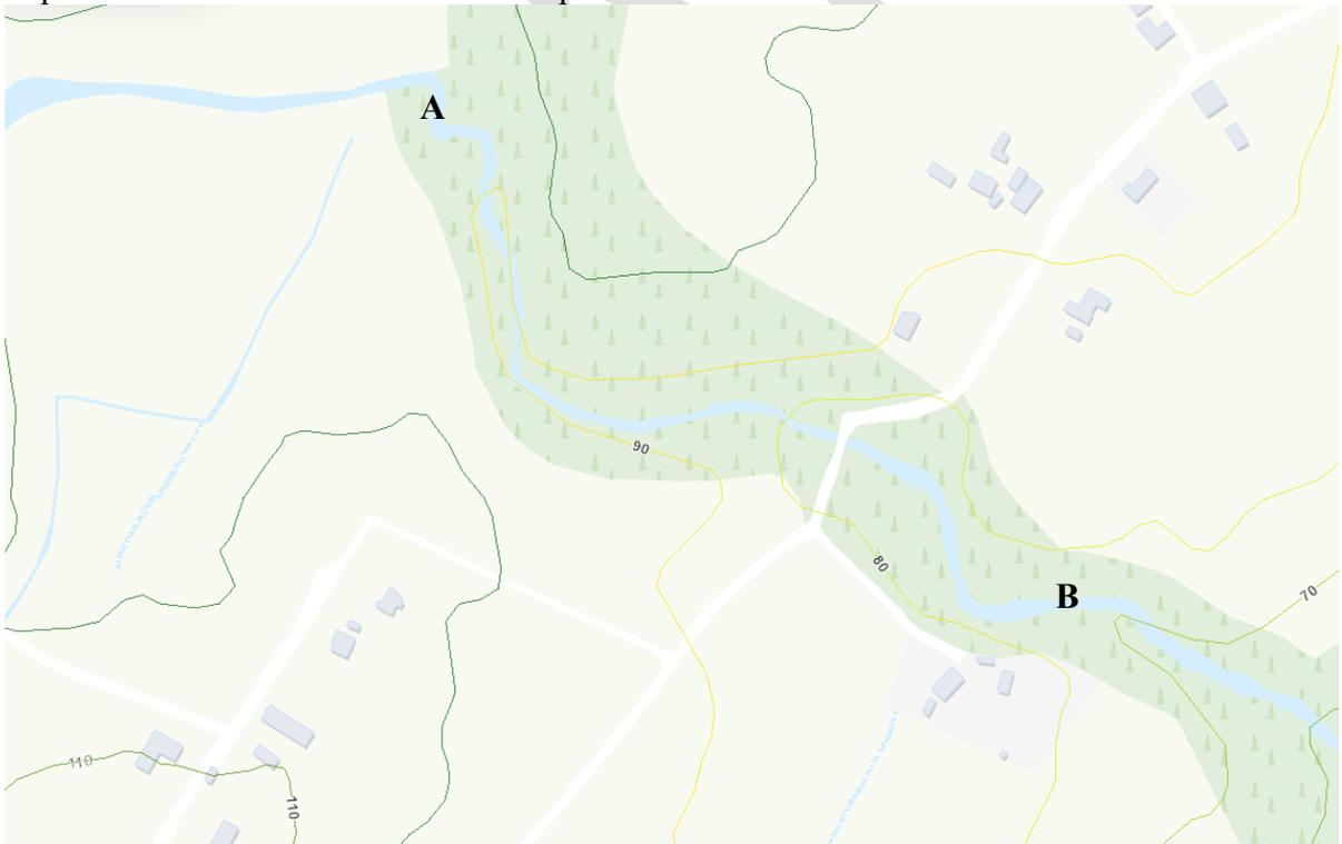
Site 2 Derryveeney. The pressure pipe will run from Point A along a fall to the turbine house at B.
