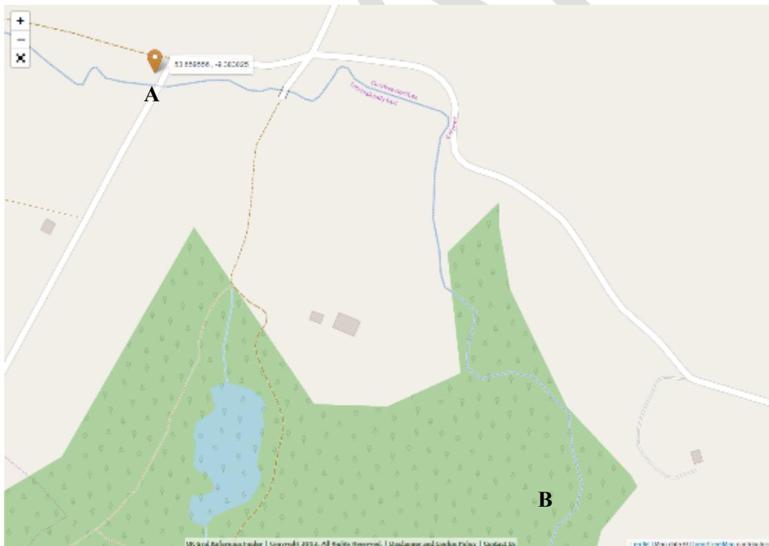
Site 1 Gortfree. The pressure pipe will run from Point A along a fall to the turbine house at B.
