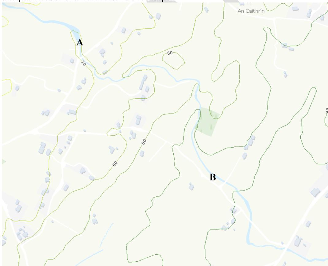
Site 3 Treanlaur. The pressure pipe will run from Point A along a fall to the turbine house at B.
