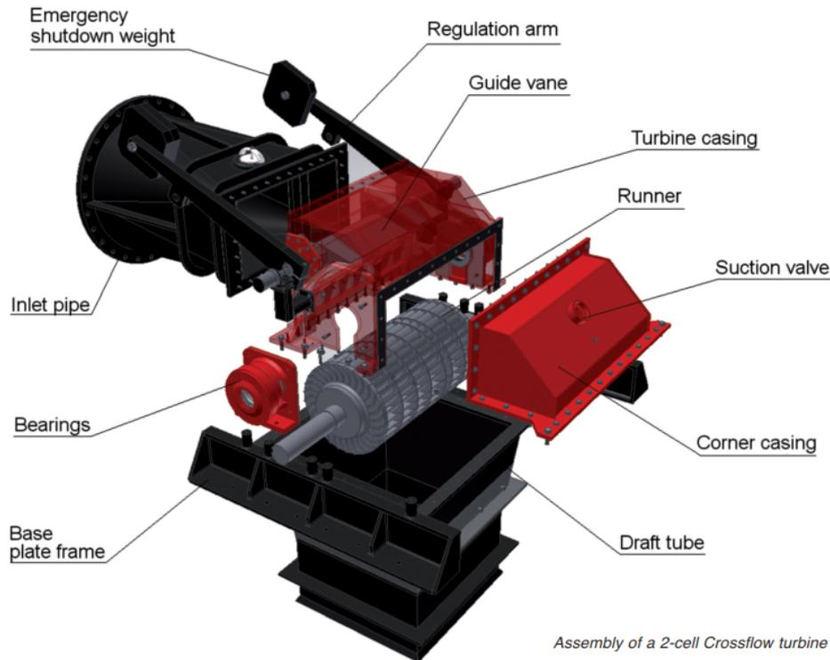
A blow up of a cross flow turbine
