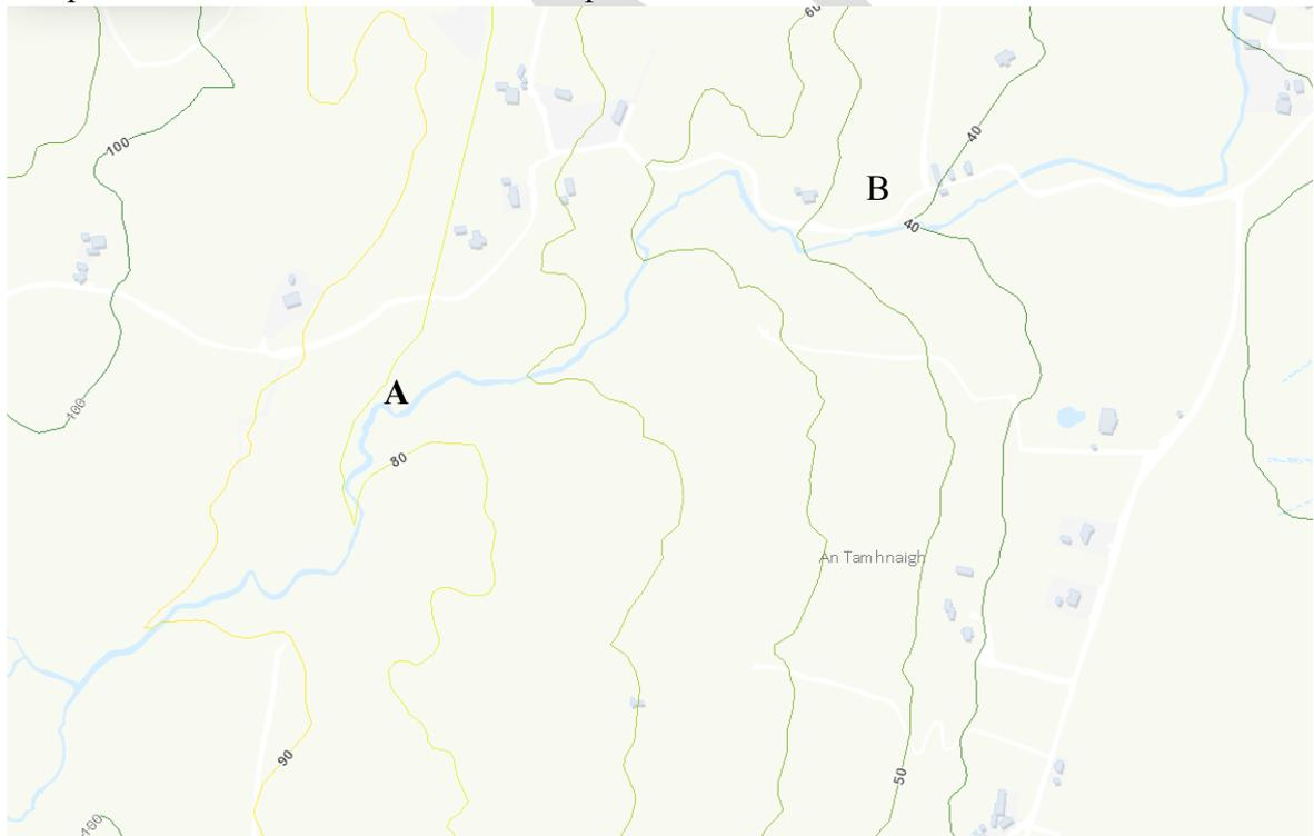
Site 4 Tamhnaidh. The pressure pipe will run from Point A along a fall to the turbine house at B.
