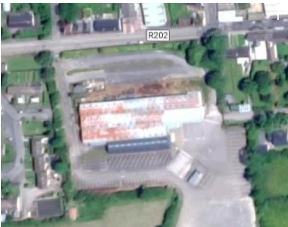
The building is facing west and is not ideally suited for roof mounted Solar PV. However, a ground mounted system could be installed and ideally orientated with a south facing solar array. The principle of achieving a net zero energy building using solar energy will require some tariff to sell export power, as it would not be feasible to match the on-site demand on a seasonal basis. Based on the data below the system is sized to optimise on-site use.
