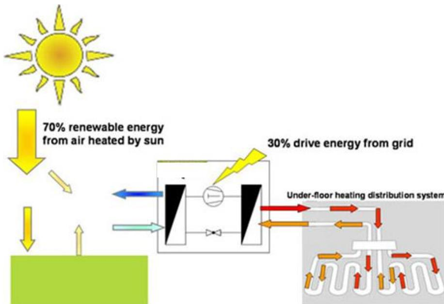
Figure 1 Air to Water heat pump for Eivers Lane Childcare
