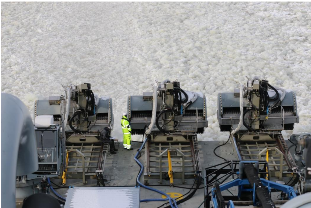
Figure 8. The large oil brush systems of the oil recovery ship Louhi. Each unit has a 4-m-wide brush system which can lift oil from ice-covered waters effectively (photo: SYKE).
