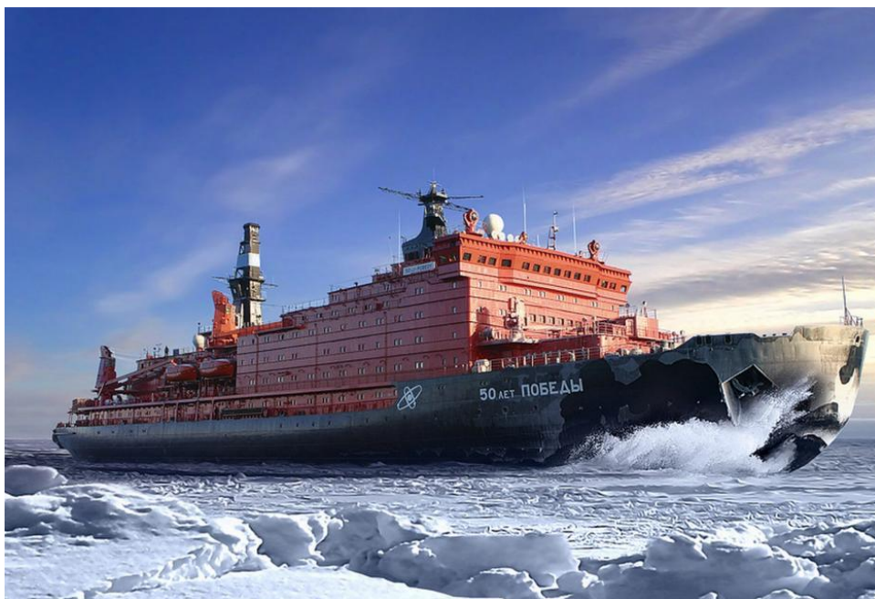
Figure 11. The world's largest icebreaker 50 Let Pobedy (50 Years of Victory) - the last of the Arktika class of nuclear icebreakers - launched in 2007 (Source: Courtesy of Rosatomflot).
