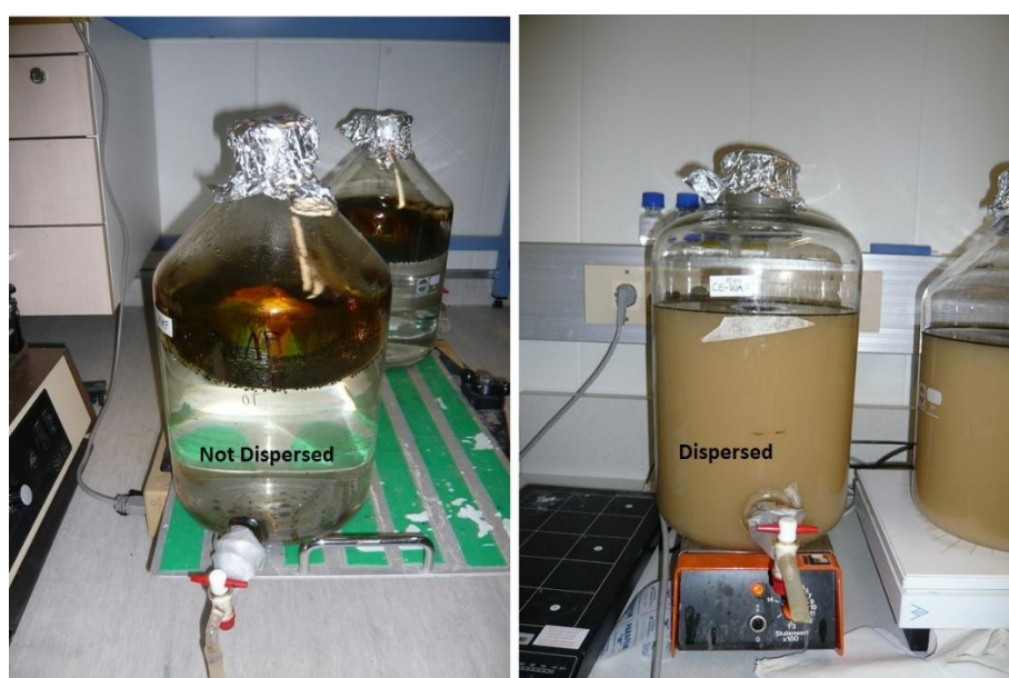
Fig 4. Non- dispersed and dispersed oil during the preparation of the water-accommodated fraction of oil for experiments with biodegradation and effects on biota in the GRACE project. (Photo K. Jørgensen).
