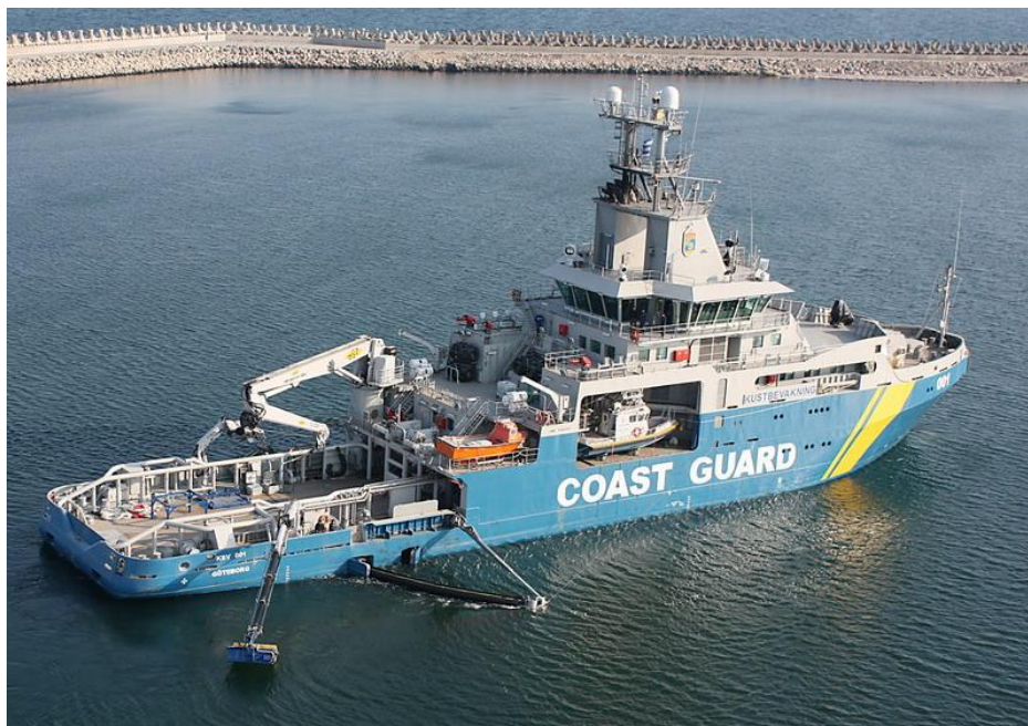
Figure 6. Oil recovery bucket and sweeping arms mounted onboard a Swedish Coast guard vessel (Photo: Lamor Ltd).
