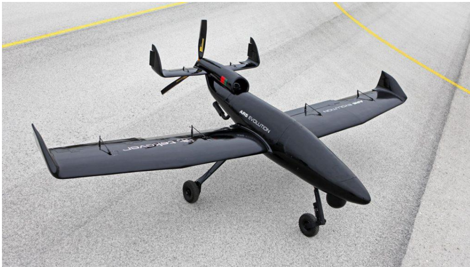
Figure 20. Tekever AR5 – a fixed wing UAS for oil spill surveillance (Rees, M. 2017).
