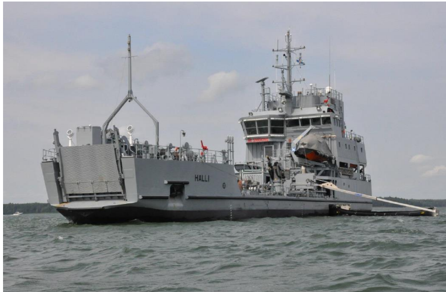
Figure 5. Finnish oil recovery ship HALLI with the inbuilt oil recovery system, inbuilt storage chamber for recovered oil and sweeping arms on both side of the hull (Photo: SYKE).
