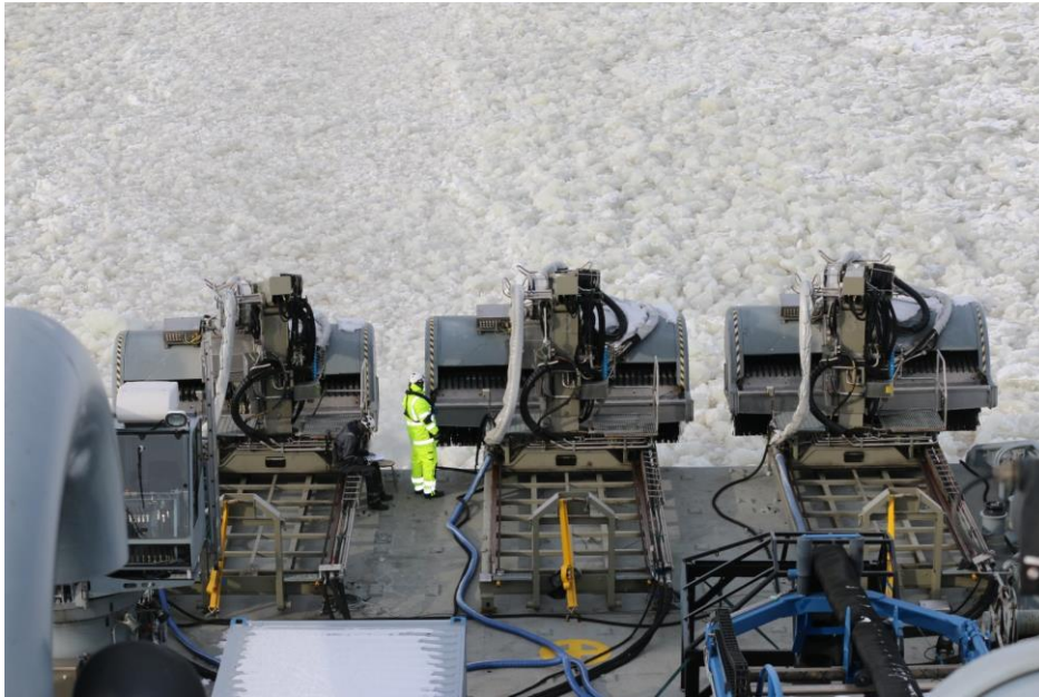
Figure 7. Robust large-scale ice brushes onboard oil recovery vessel LOUHI during the Oulu Ice Trial in 2016. These ice brushes have been designed for oil recovery in ice. (photo: SYKE)
