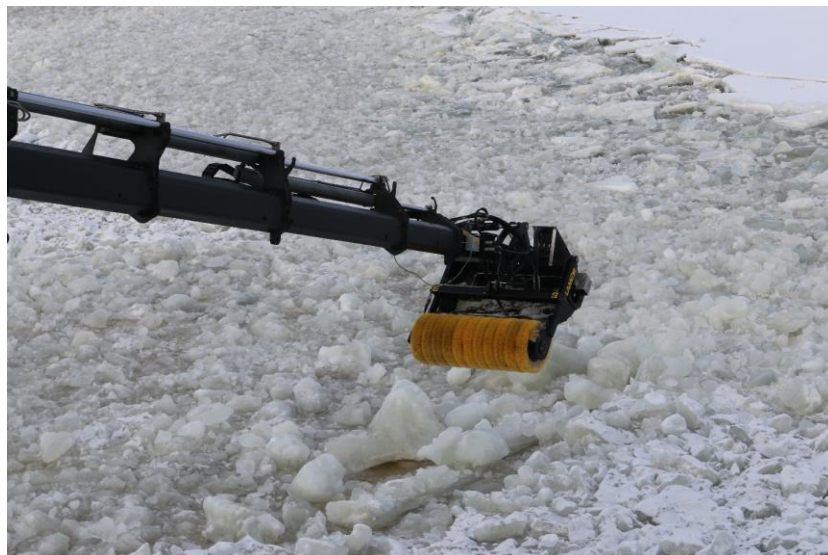
Figure 6. A brush type bucket skimmer designed for oil recovery among ice. (Photo: SYKE)
