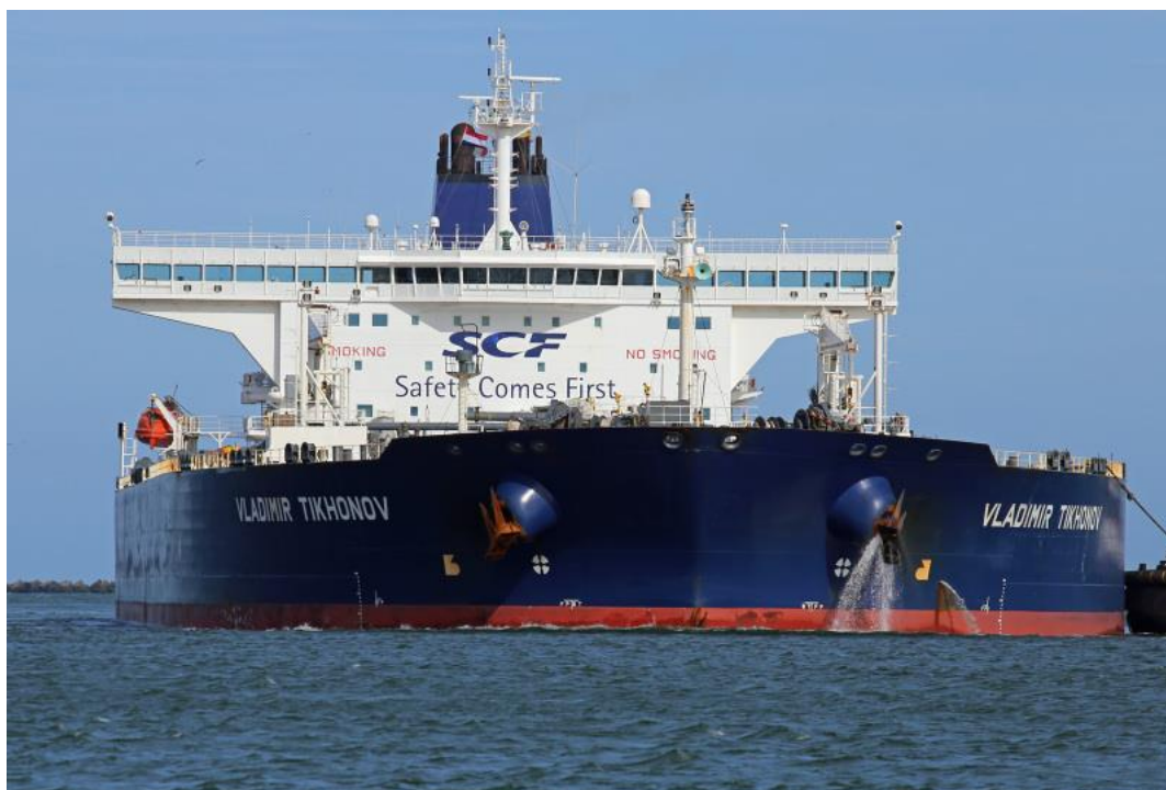
Figure 6. During 2011 a new route north of the New Siberian Islands was established, where the water is deep enough to accommodate tankers with draughts of over 12 metres, and for the first time in history the route was navigated by the Sovcomflot tanker Vladimir Tikhonov, a Suezmax ice class 1A vessel with a dead weight of over 160 000 tons (AKER 2012) (Photo: D. Sands).
