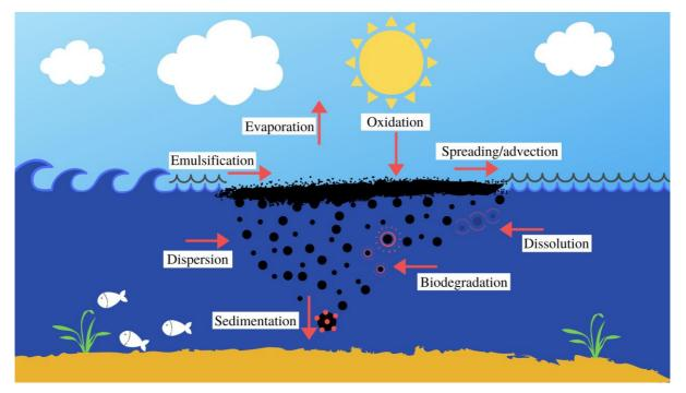
Fig. 2 - Physical and chemical processes known as weathering of oil.
