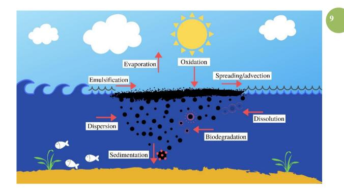
Figure 3 – Oil weathering processes
