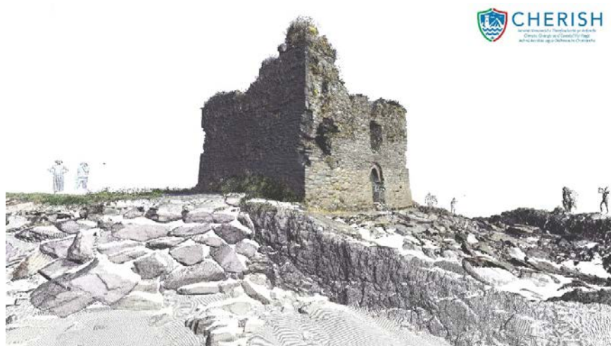
Figure 25: 3D point cloud captured using Faro Focus 120 Laser Scanner
