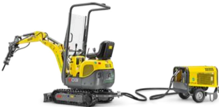
Figur 23: Dual-drive gravemaskin (Wacker Neuson, 2016a).
