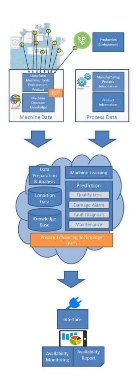
Data will be gathered using sensors located on the machines and tools. **Additional information** will be collected from the manufacturing environment, the product itself as well as the machine operator's experience.
