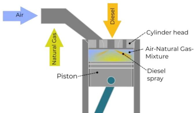
Figure 1: DUAL FUEL ENGINE (Diesel-cycle)
