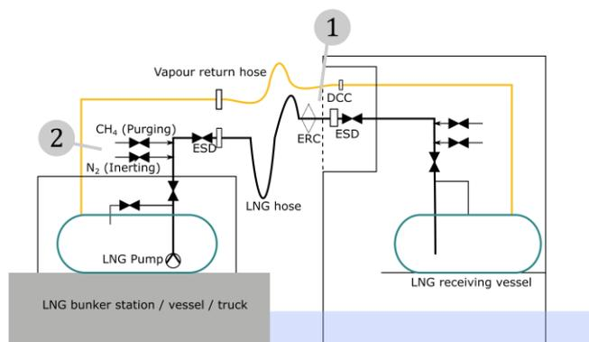
Figure 7: Bunkering scheme
