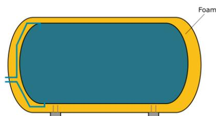
Figure 4: Pressure tank - foam insulated
