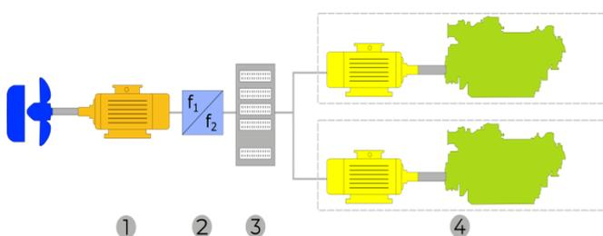
Figure 1: Setup of a diesel-electric drive train
