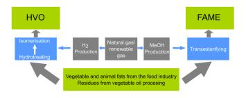
As it can be seen within the graphic illustration, the process of HVO production differs from the production process for biodiesel (FAME), as it is a catalytic process with hydrogen (hydrogenation); compared to the esterification process used for FAME production.
