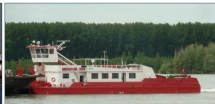
Type 3 pusher: 2 x 1185 kW/1000rpm
