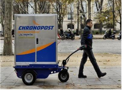
Image 45: Manually-controlled Chronocity vehicle<sup>22</sup>
