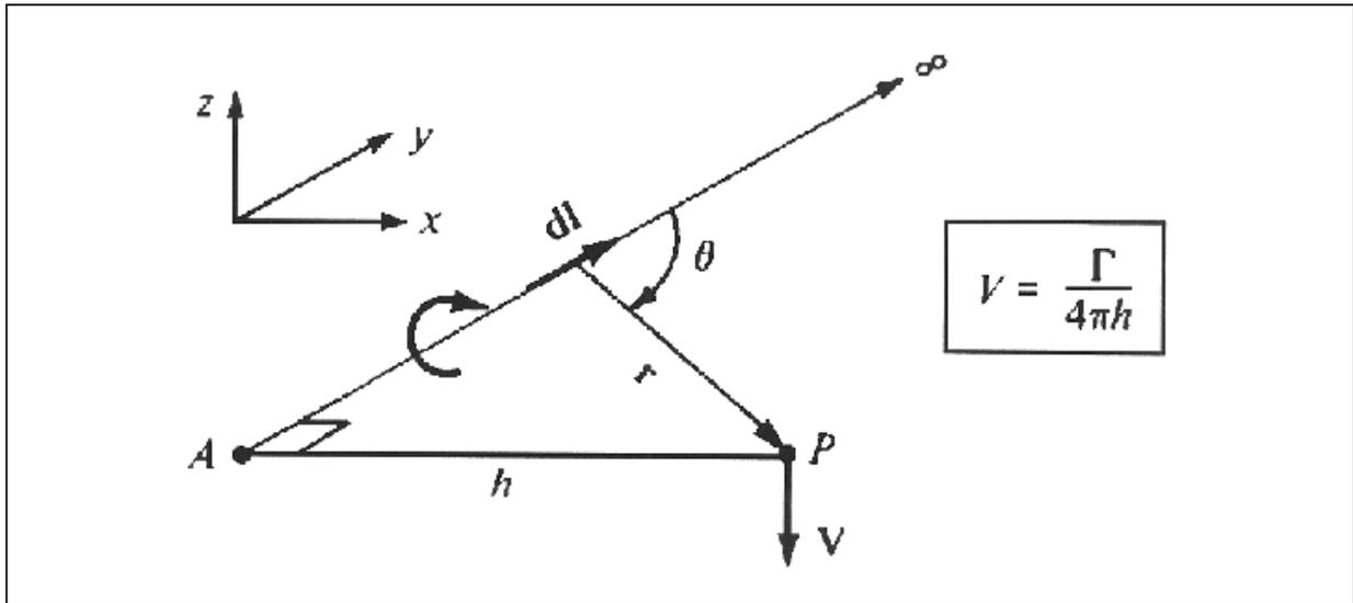
Velocity contribution to flow field at wing location orthogonal to free flow direction ! Always vertical for a planar wing (worst situation)
