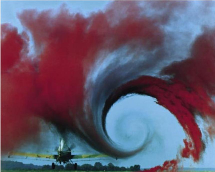
Power is also required for the kinetic energy in vortices → keep velocity in vortices low for low power consumption
