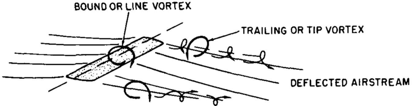
$\Gamma$  orthogonal to incoming free flow  $\rightarrow$  lift      sectional lift  $\sim \Gamma \cdot v$
