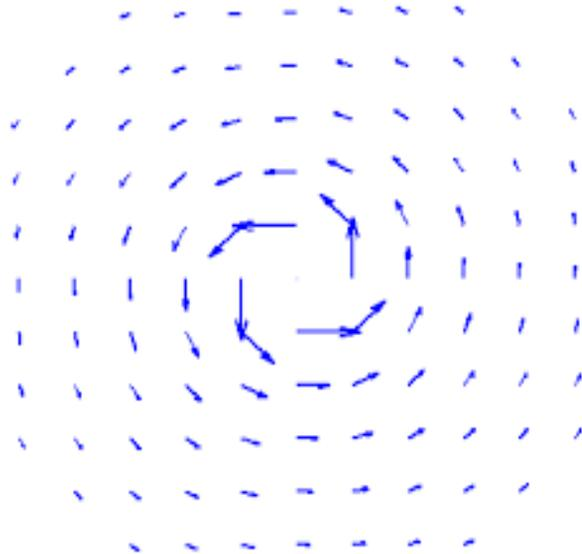
Air flows in circles around a (thought) axis -> vortex filament
