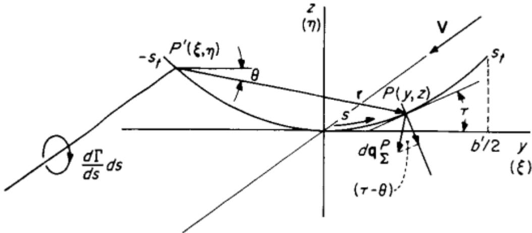
Munk: best, if component normal to local wing section is  $w_0 \cdot \cos(\tau)$ ,  $w_0$  being constant over wing span, then minimum total induced drag
