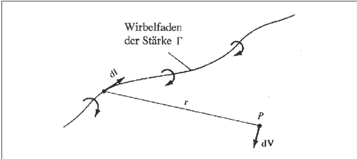
vortex filament = electric current
