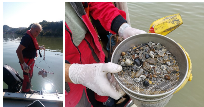
Bottom sediment sample collection and sieving in the field.
