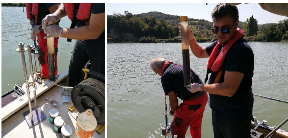
Bottom sediment sample collection and sieving in the field.
