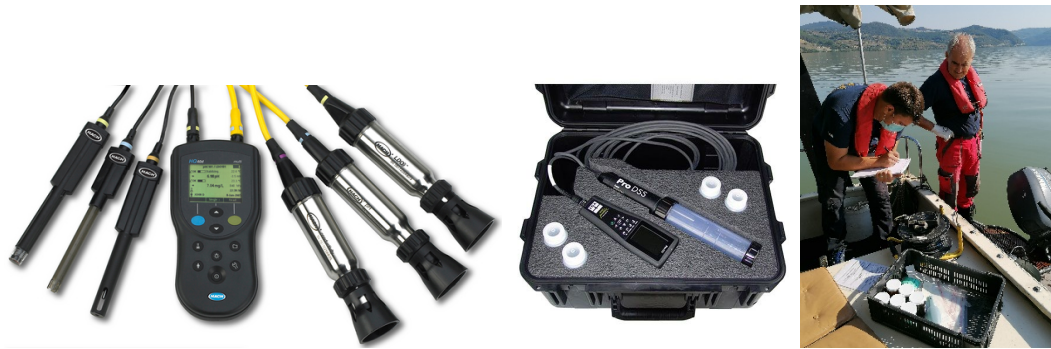
Multiparameter probes used and the measurement of in-situ water quality parameters.
