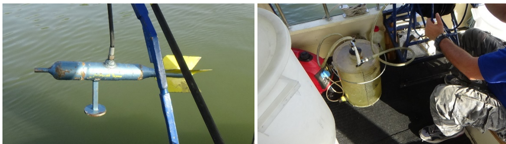
Collection of suspended sediment samples.
