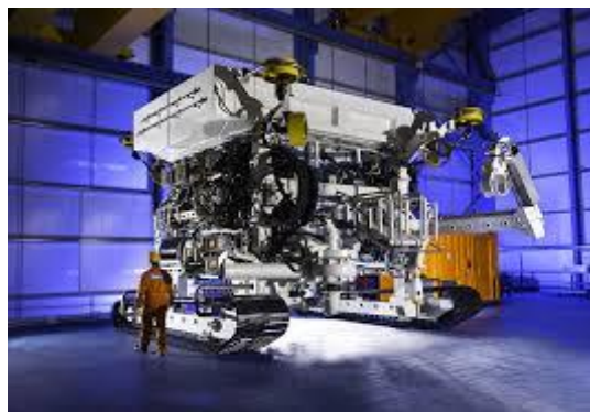
FIG 8: Ejemplo ROV de oruga y arado ( https://www.smd.co.uk/wp-content/uploads/2018/05/QTrencher-1600.pdf )
