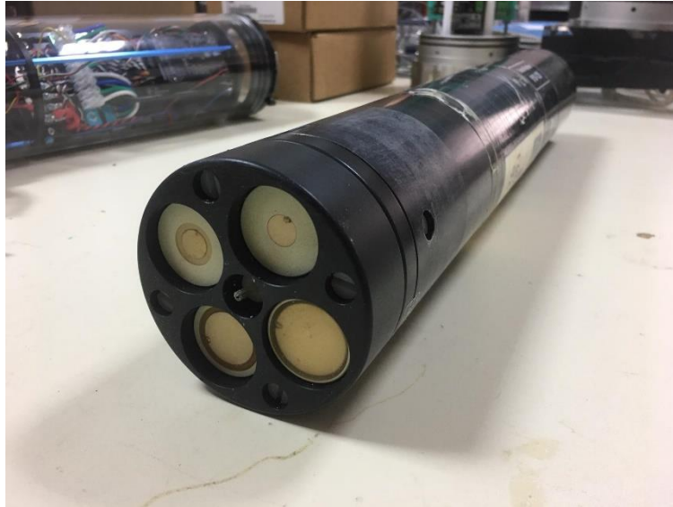
FIGURA 16 - ACOUSTIC BACKSCATTER SYSTEM, AQUATEC AQUASCAT 1000s
