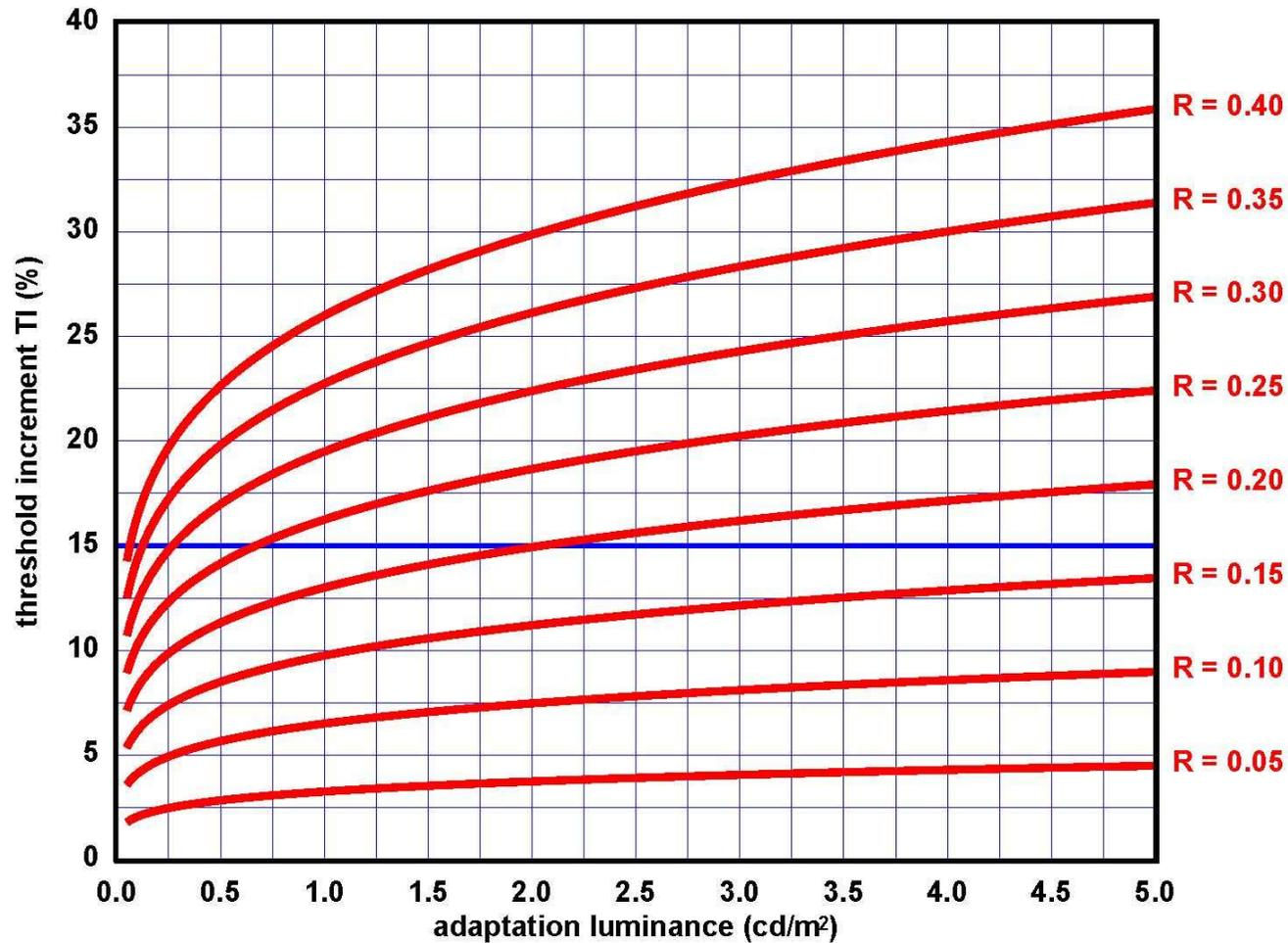
Threshold increment as function of adaptation luminance for different ratios R of veiling luminance to adaptation luminance
