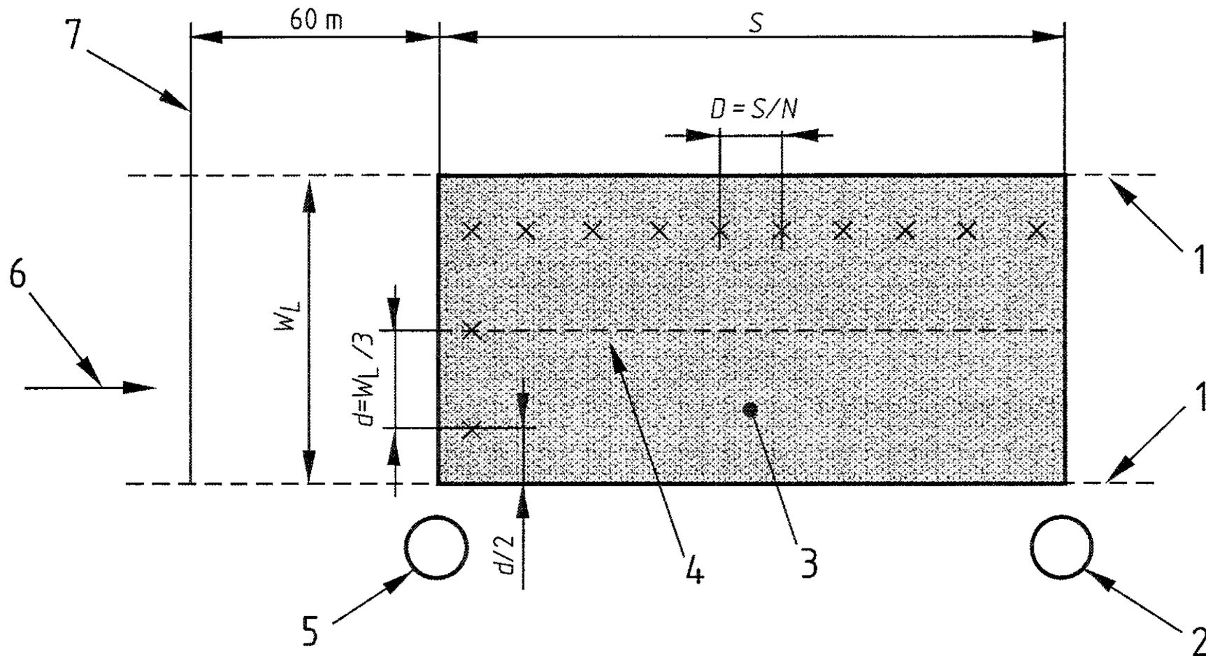
1 ... Edge of lane, 2 ... Last luminaire, 3 ... Field of calculation, 4 ... Centre line of lane,
