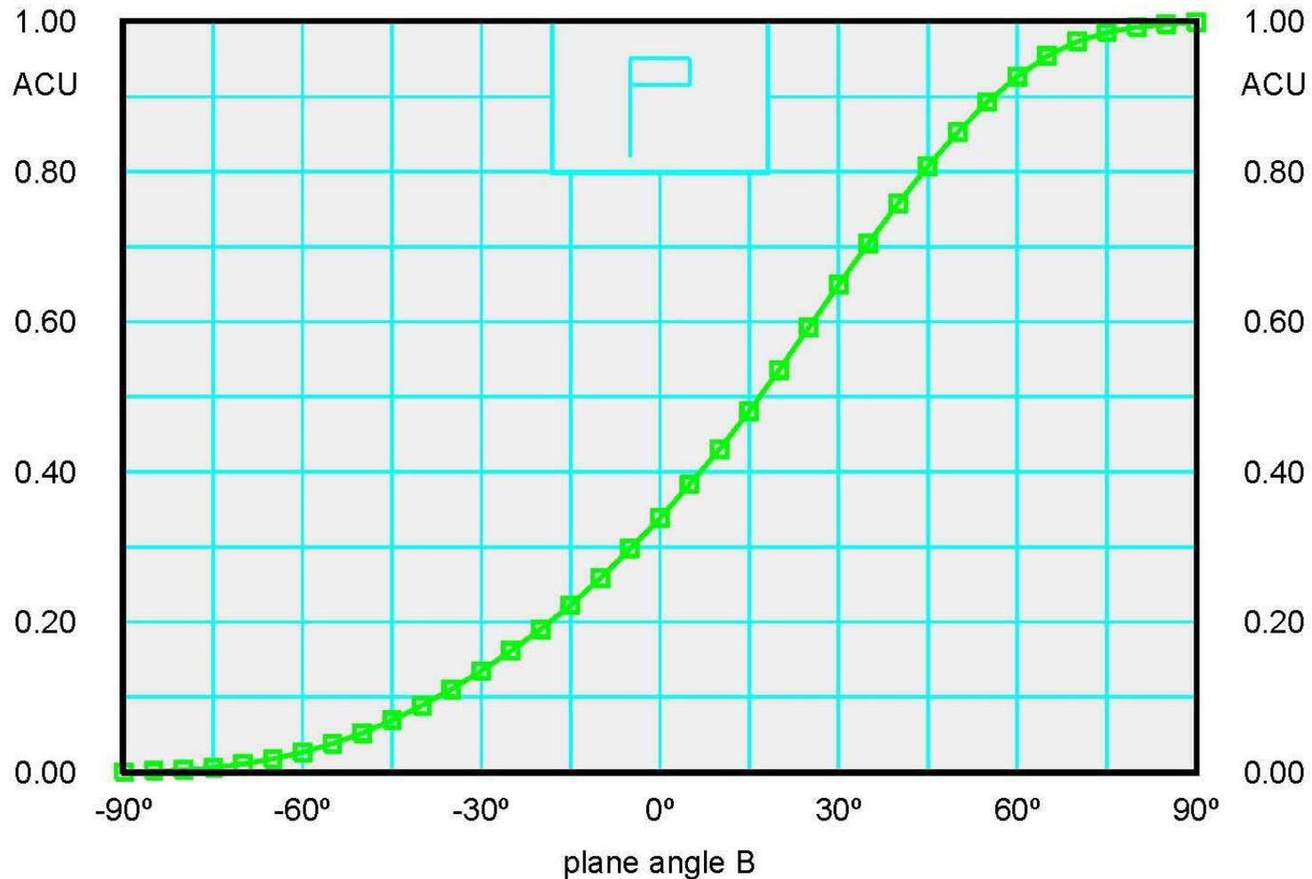
Accumulated utilances road lighting as function of plane angle B from  $-90^{\circ}$  to  $+90^{\circ}$
