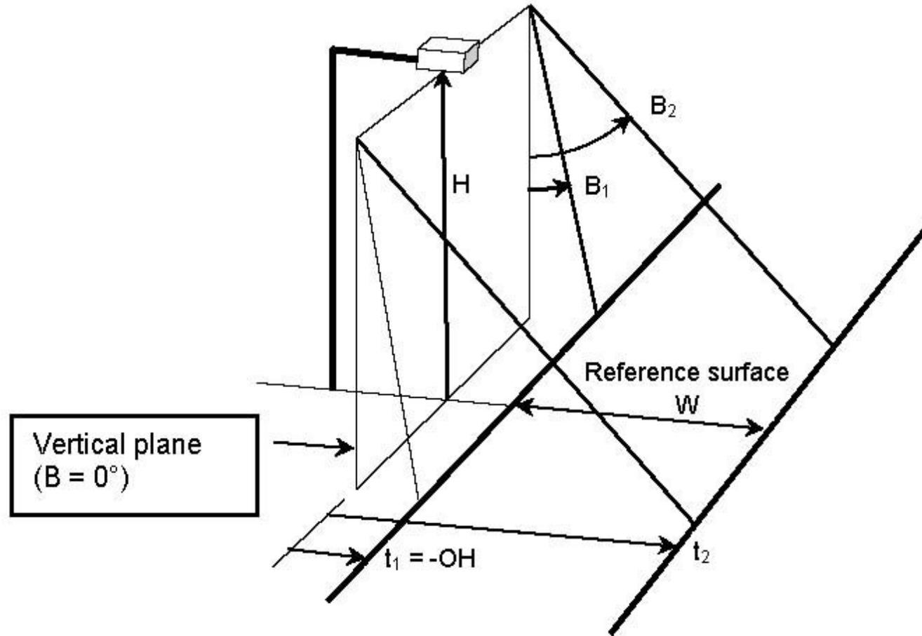
$O_v$  overhang (m);  $W$  width of reference area (m);  $H$  luminaire mounting height (m);
