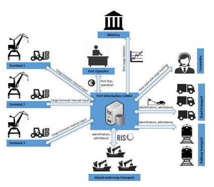
26. Figure: Planned functional structure of the pilot system (Source: RSOE)
