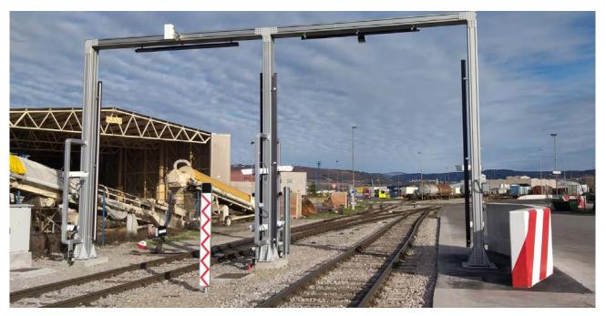
Figure 3: installed OCR system in the port of Koper (Source: Luka Koper's archive)
