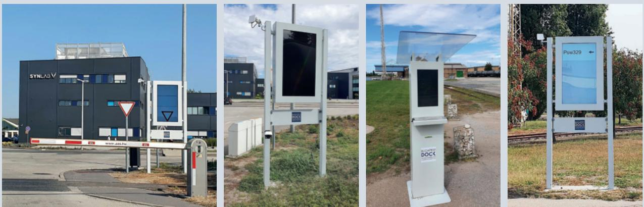
*Elements of the smart traffic management system: Access control at the gates, smart info panel with license plate recognition camera, InfoPoint (kiosk) and smart signpost*
