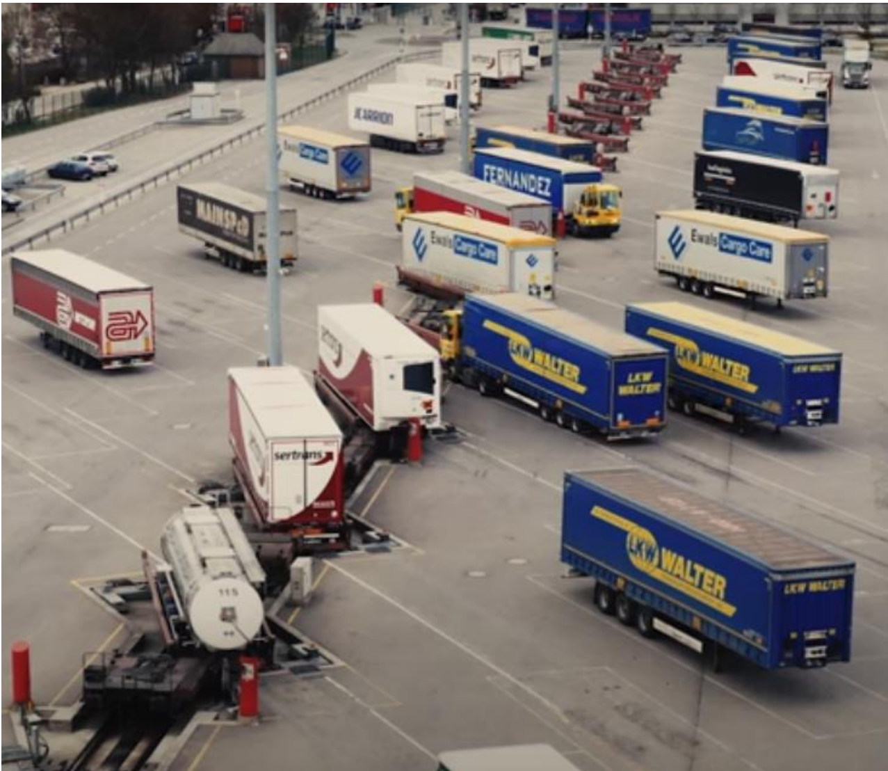
Figure 19 Train loading with the LOHR system (source: Efficient LOHR Railway System (timelapse) https://www.youtube.com/watch?v=MTvSOrTXFzw )
