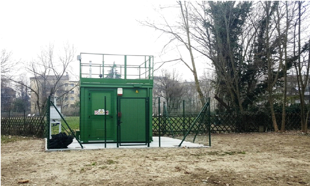
Figure 4.2 - The reference monitoring station in Parco Cittadella (background site) inside Parma urban area.
