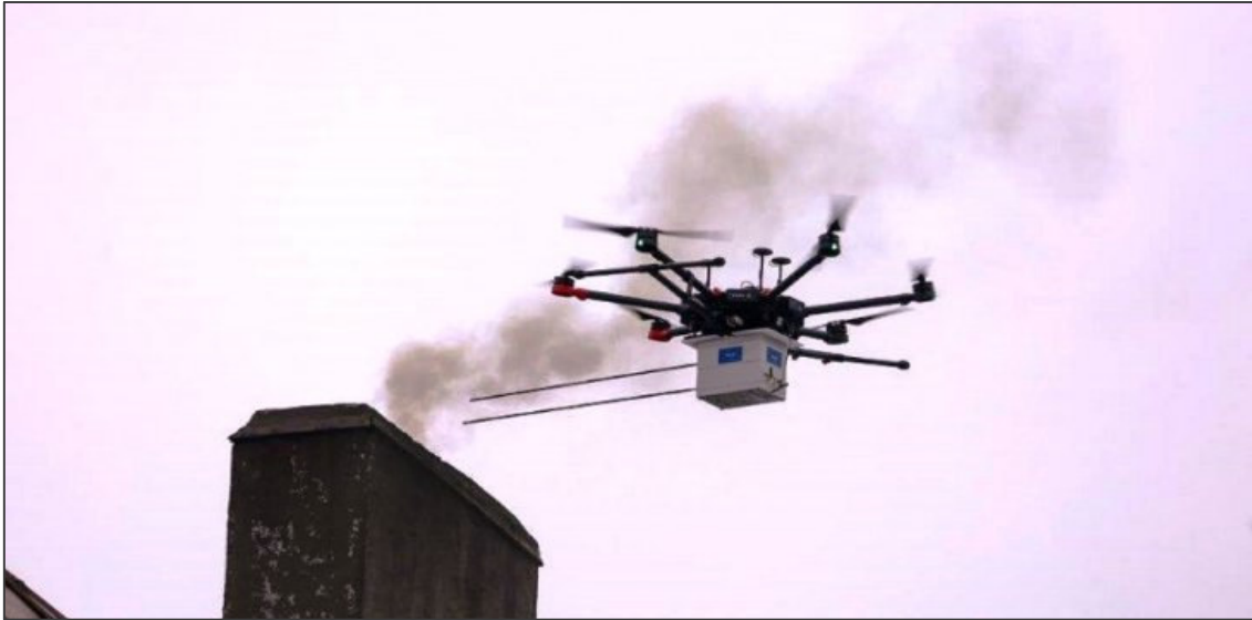
Figure 6.7. Example of use of air quality sensor system installed on drones
