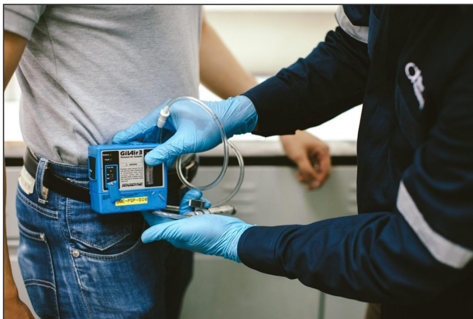
Figure 6.4. Example of use of air quality sensor system for personal monitoring
