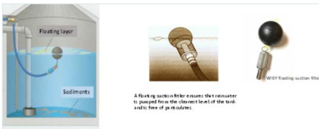
Figure 8: Floating device with a suction pump delivering water to the different points of use.
