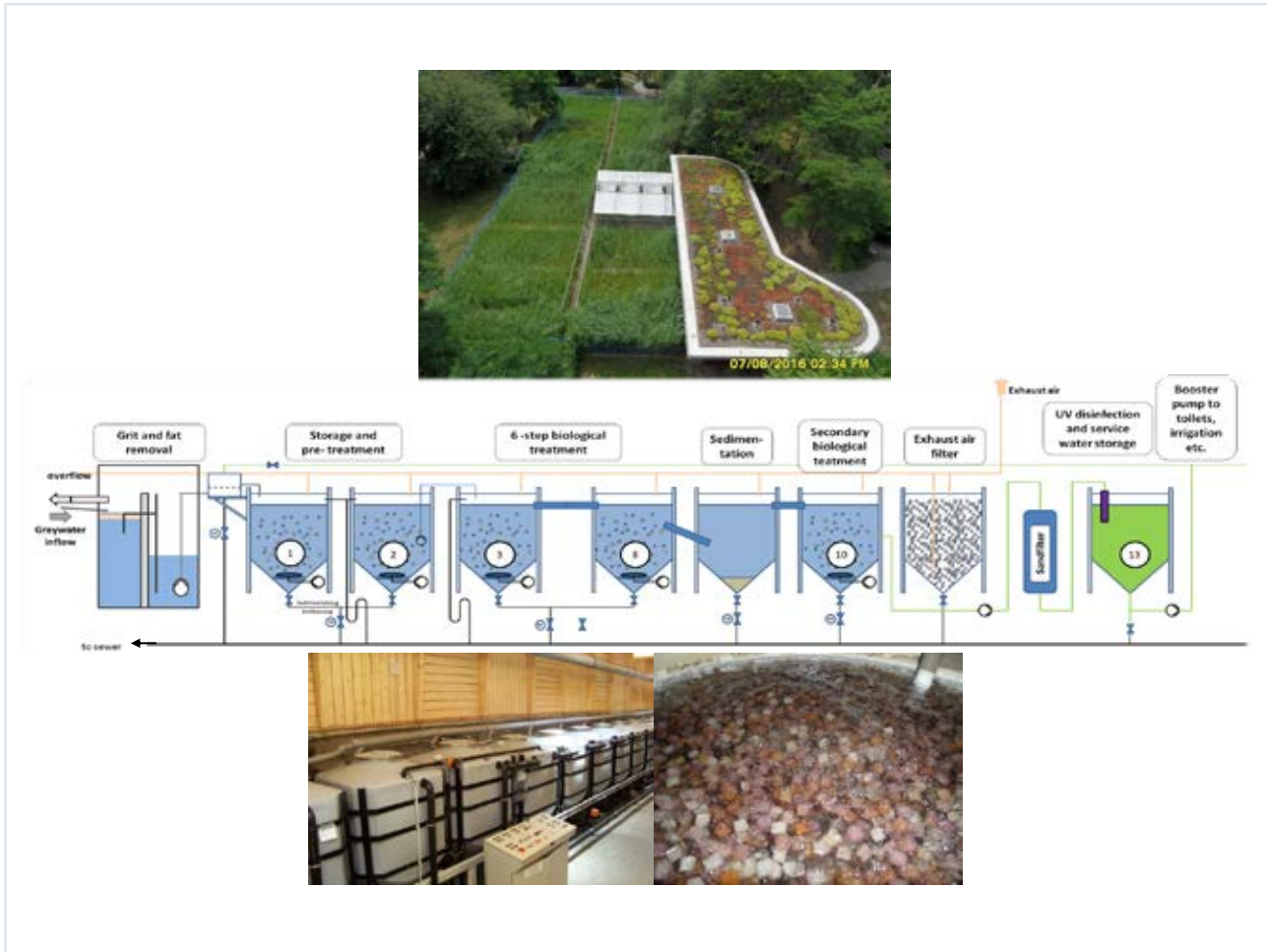
Figure 21: The so-called “water house” containing the greywater recycling system (above) and a schematic diagram of the different MBBR treatment stages. The aerated MBBR with carrier media (below right).
