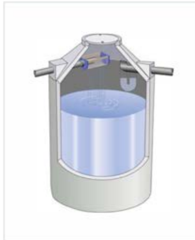
Underground concrete cistern (3 - 12 m 3 ) (Mall)
