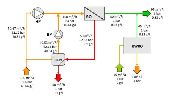
*Fig. 4*). This brackish water could be desalinated with a brackish water reverse osmosis (BWRO) system (see *Fig. 5*), which will be modelled by using Q+ software [45].
