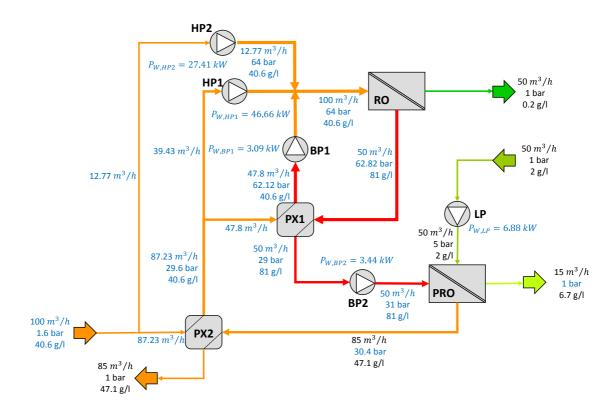
Fig. 7. Results for the second configuration of the patent. Black values are taken directly from the patent and blue values are calculated.
