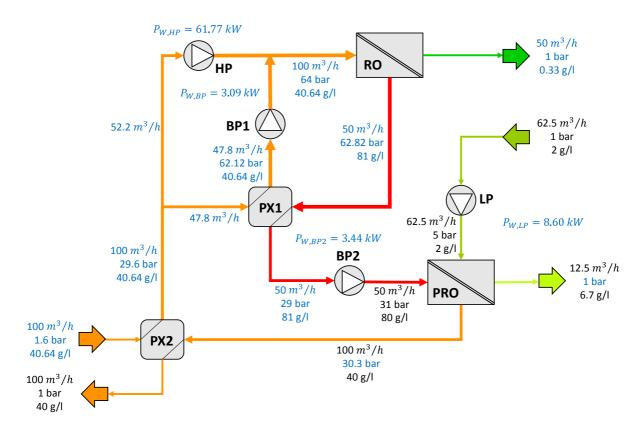
Fig. 6. Results for the first configuration of the patent. Black values are taken directly from the patent and blue values are calculated.
