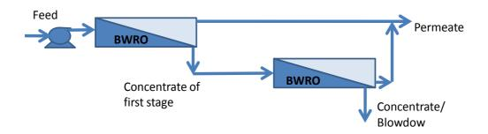
Fig. 5. Basic configuration of a BWRO desalination system.
