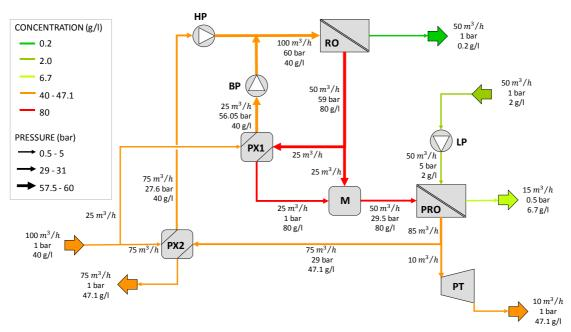
Fig. 3. Schematic diagram of the third SWRO+PRO arrangement proposed in the patent.
