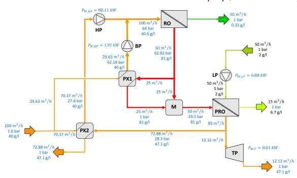
Fig. 8 shows the results for the third configuration of the patent where the second booster pump BP2 has been replaced by a mixer and part of the diluted PRO draw solution is sent to a Pelton turbine for power generation.
