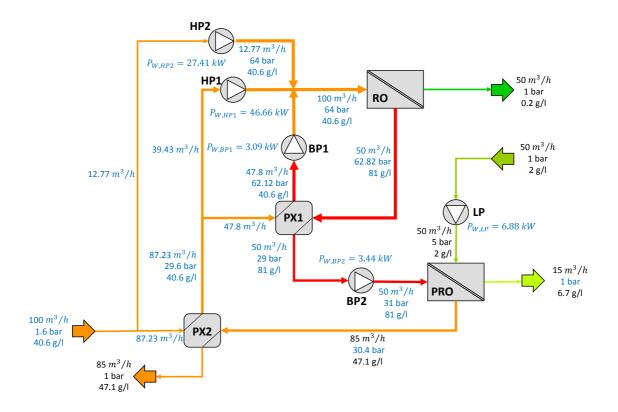
Fig. 7 depicts the results related to the second RO-PRO configuration. Note that in this scheme, there are two high-pressure pumps in the RO, with power consumption of 46.6 kW and 27.4 kW, for HP1 and HP2 pumps, respectively.
