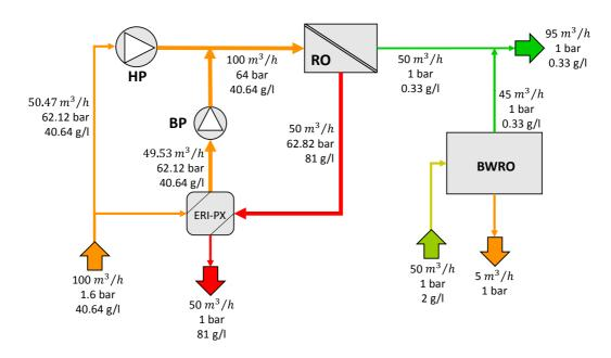
Fig. 4. Base case configuration of the SWRO desalination process without PRO and with BWRO depicted as a black box (see Fig. 5).
