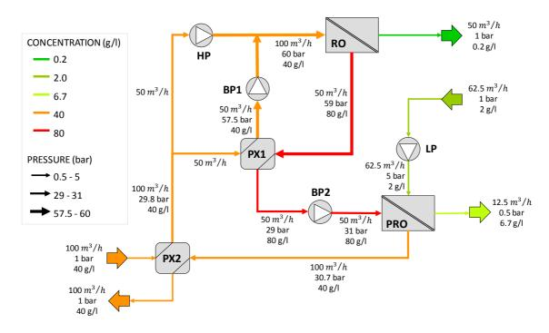
Fig. 1. Schematic diagram of the first SWRO+PRO arrangement proposed in the patent analysed.
