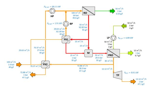
Fig. 8. Results for the third configuration of the patent. Black values are taken directly from the patent and blue values are calculated.
