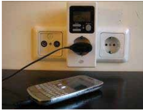
Figure 20-1: Measuring electricity consumption of electric appliances
