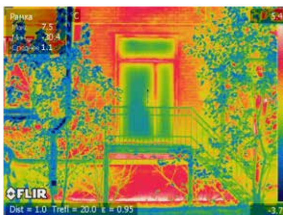
Figure 47-2: Heat leakage through the joints of walls and improperly installed door unit
