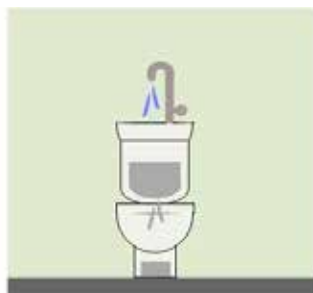
Figure 58-12: Sketch of a toilets with washbasin insert. Principle sketch after an idea, recommended in Cape town
