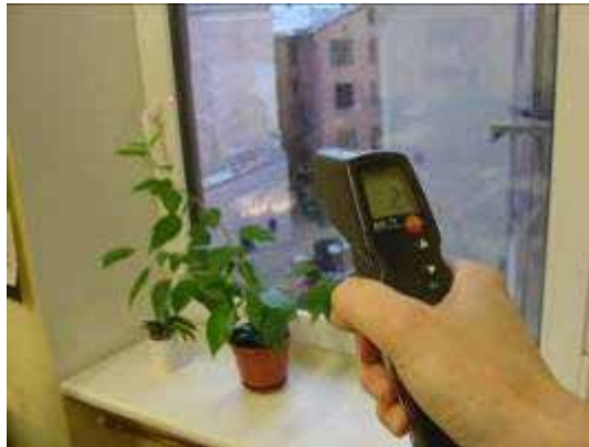
Figure 20-4: Detecting thermal bridges with an infrared thermometer
