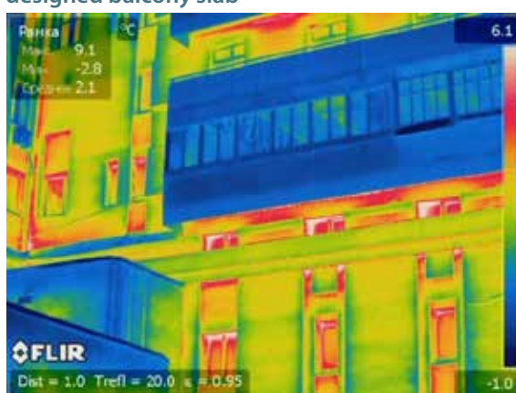
Figure 47-5: Heat leakage through the joints of walls and improperly designed balcony slabs
