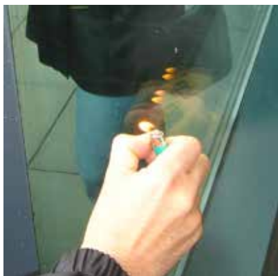
Figure 39-5: The picture shows the reflection of the light, which is darker and more reddish: this means that the window is coated.
