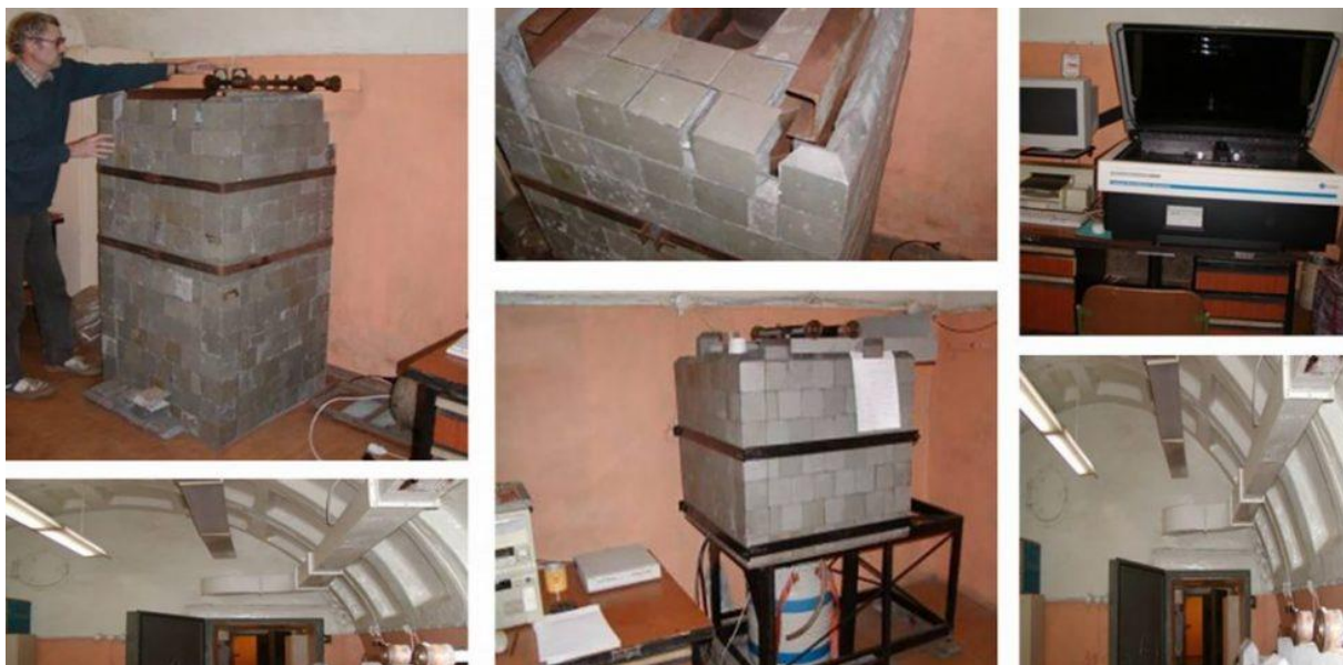
Figure 1: Underground rooms with gamma spectrometer and Low Activity Liquid Scintillation Analyzer in Khlopin UL.
