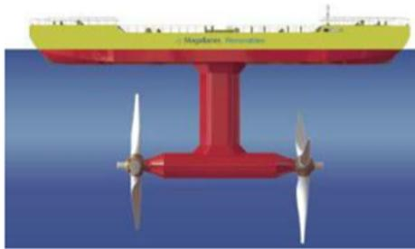
Figure 6: Schematic of the Magallanes ATIR tidal stream device.
