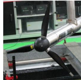
Figure 7: Scaled Magallanes ATIR turbine model used in laboratory testing.
