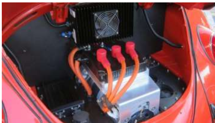
Fig. 3.4 Over 50V installation marked orange, source: www.e-auto.guru
