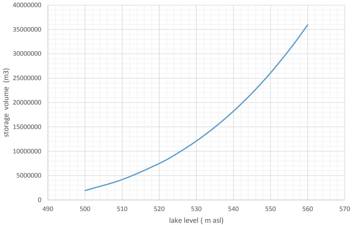
Figure 4. Reservoir storage curve for the Ridracoli dam.
