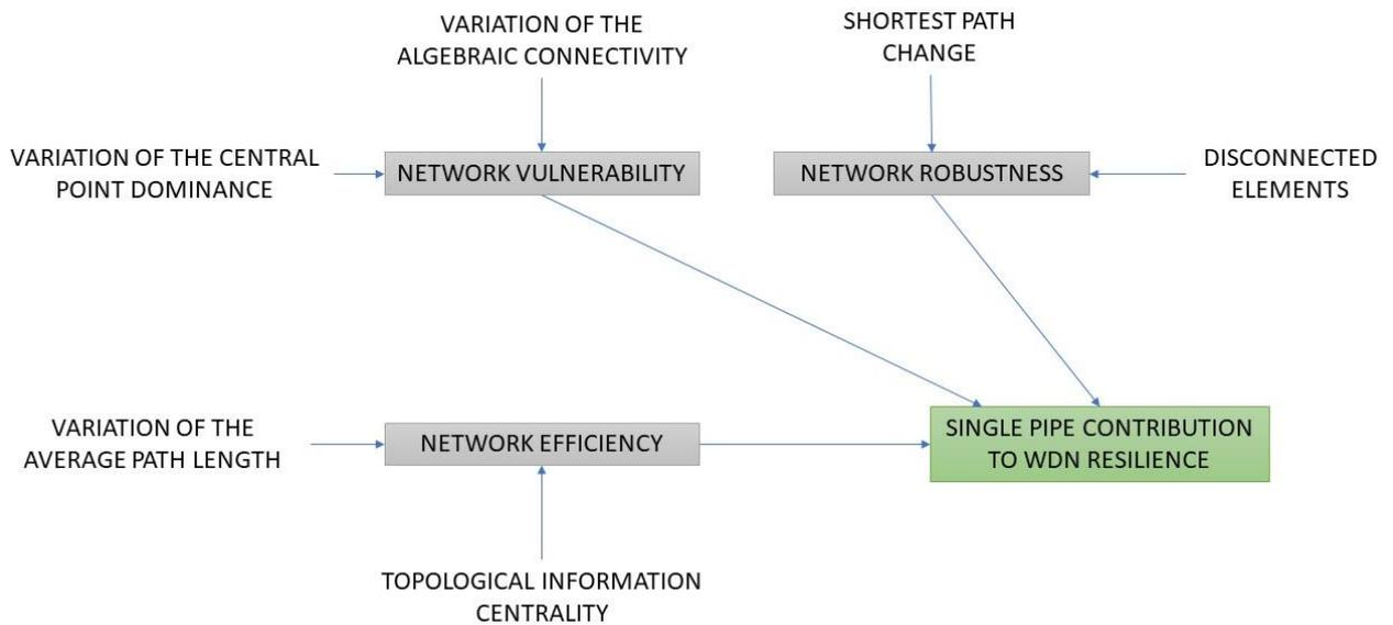
*Figure 13. Structure of the aggregation of the GT metrics for assessing the individual pipe contribution to WDN resilience, to be performed using BBN.*
