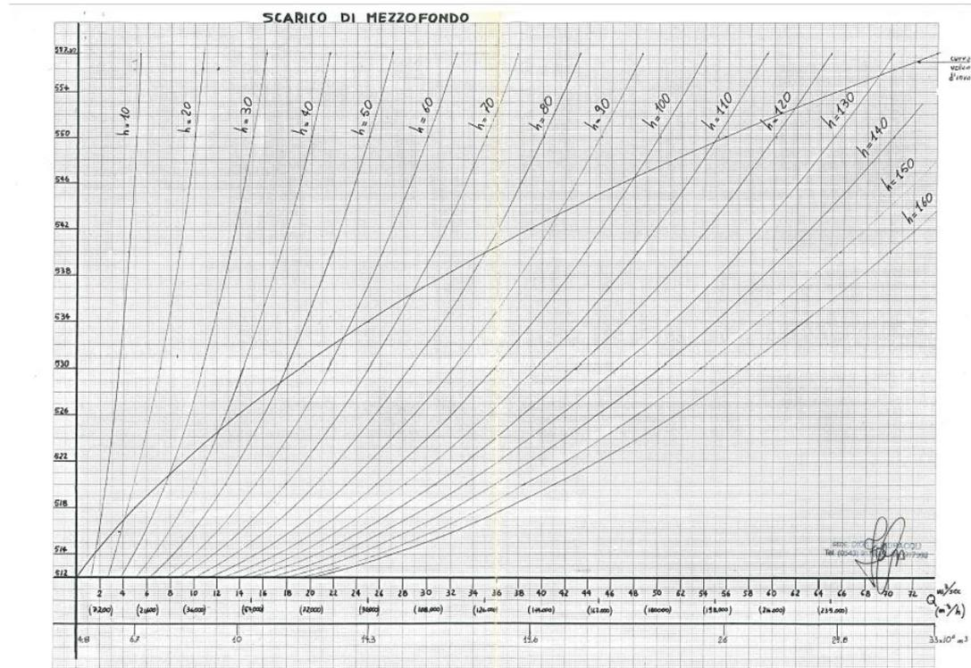
Figure 2. Outflow curves for the middle bottom outlet of the Ridracoli dam (source: Romagna Acque).
