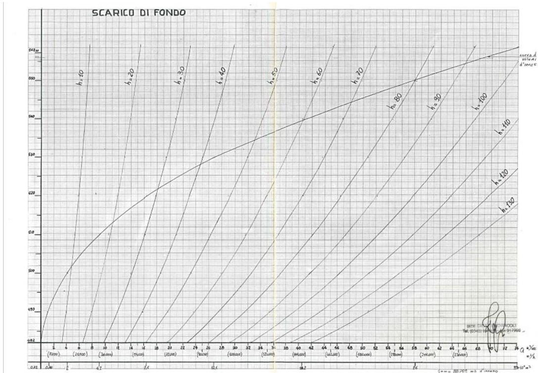
Figure 1. Outflow curves for the low bottom outlet of the Ridracoli dam (source: Romagna Acque).
