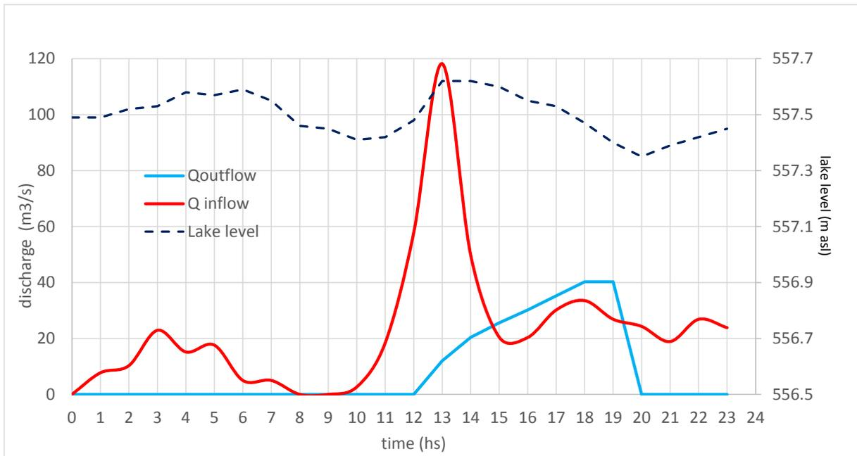
Figure 5. Flood event occurred on December 2010, Ridracoli dam: reconstruction of the inflow hydrograph. The outflow hydrograph and the recorded lake level are also shown.
