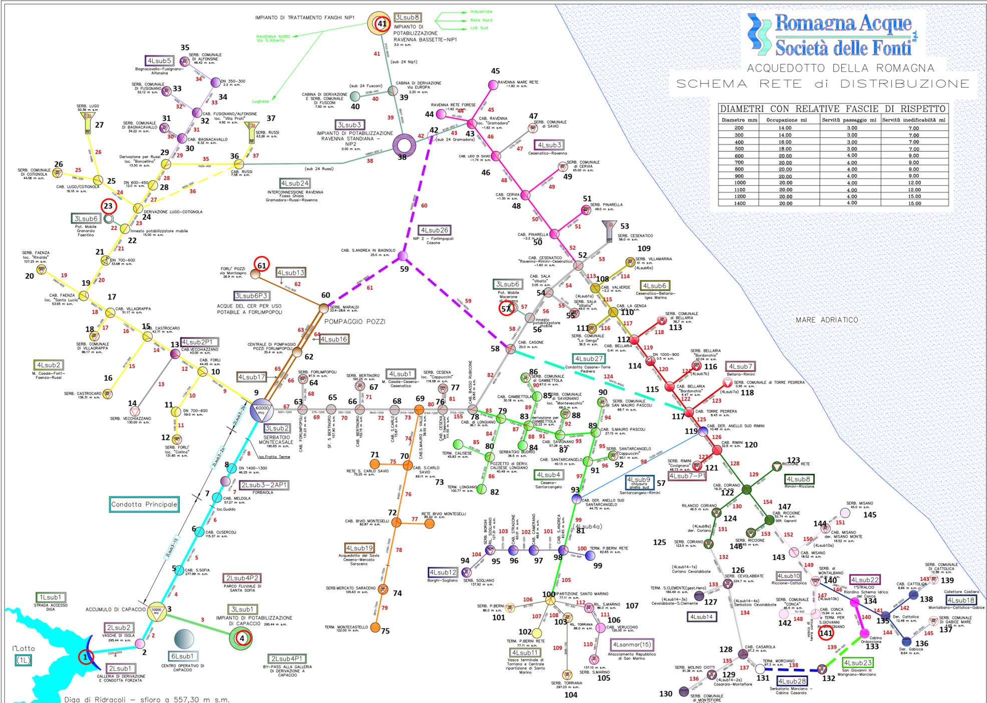
*Figure 12. Topological Scheme of the drinking water supply system managed by Romagna Acque*
