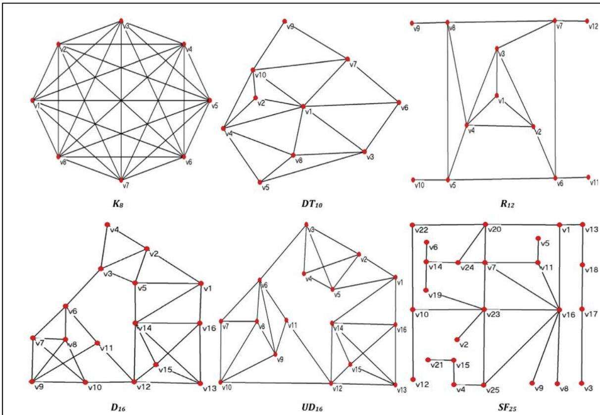
Figure 11. Comparison of the topology of different hierarchical (above) and distributed (below) networks (Yazdani et al., 2013)
