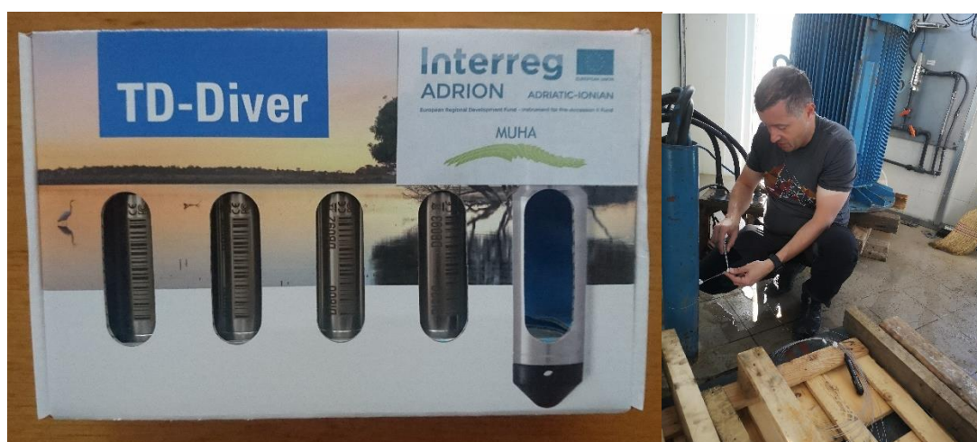
Figure 2 Automatic groundwater loggers - Automatic groundwater loggers CTD-DIVER 100m (9 pieces), Barometric pressure loggers (4) and Logger programming unit (1)
