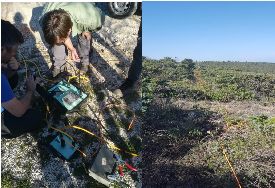
Figure 3 Geophysical research (geoelectric tomography method)
