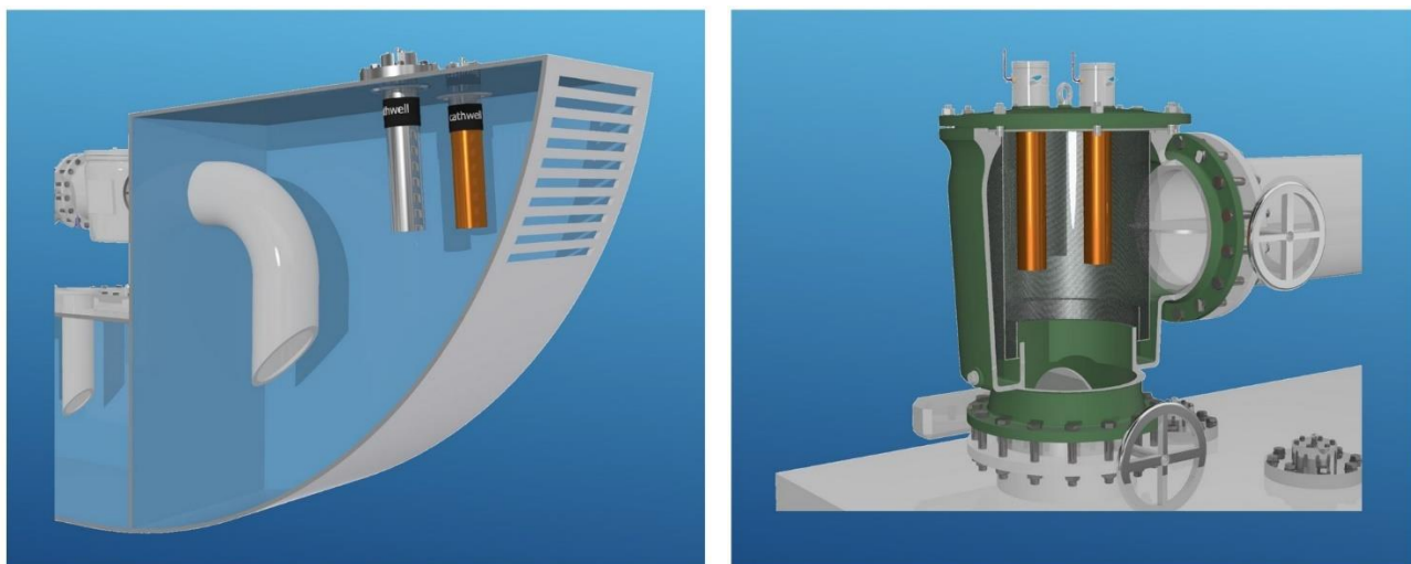
Figure 25: MGPS and ICAF anodes mounted in sea chests to prevent fouling and corrosion (left); MGPS/ICAF anti-fouling anodes mounted at strainer lid (right) [16]
