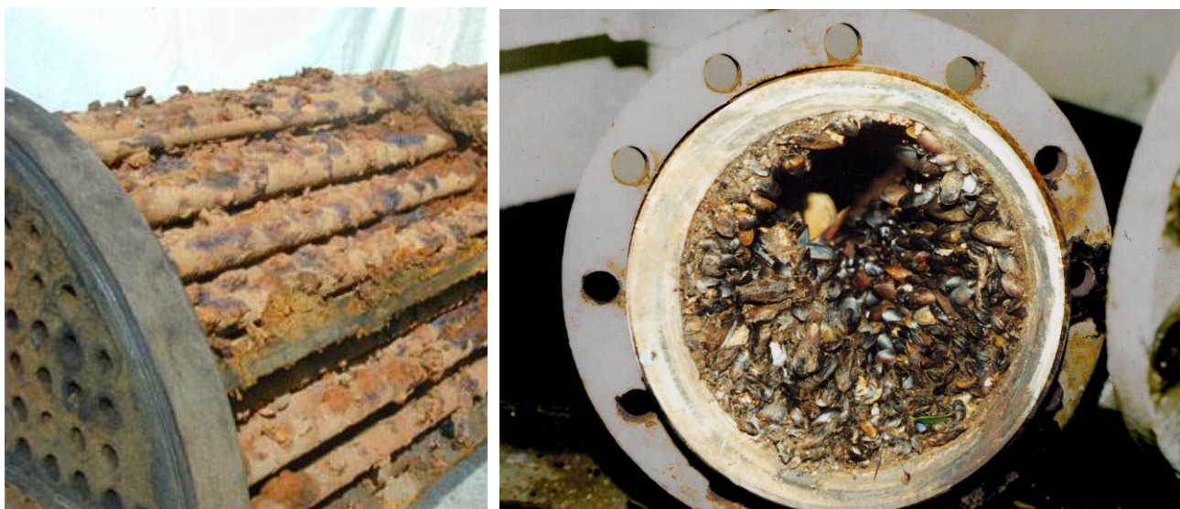
Figure 21: Problems of corrosion and bio-fouling of pipes and heat exchangers in contact with seawater [7] [8]
