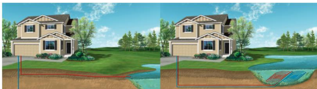
Figure 2: Open (left) and closed (right) version of the seawater heat pump system [1]
