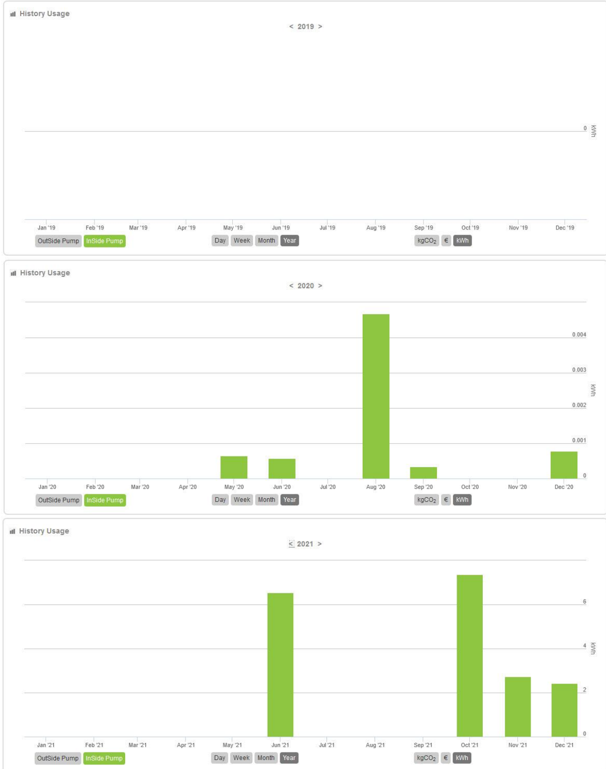
Figure 19. Diagram of monthly power usage (in kWh) of Pump C1 (Years 2019 to 2021).
