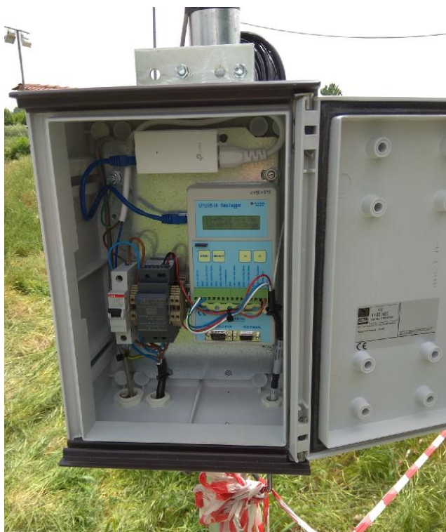
Figure 27. Data logger (left) installed next to the borehole well and submersible sensor (right)
