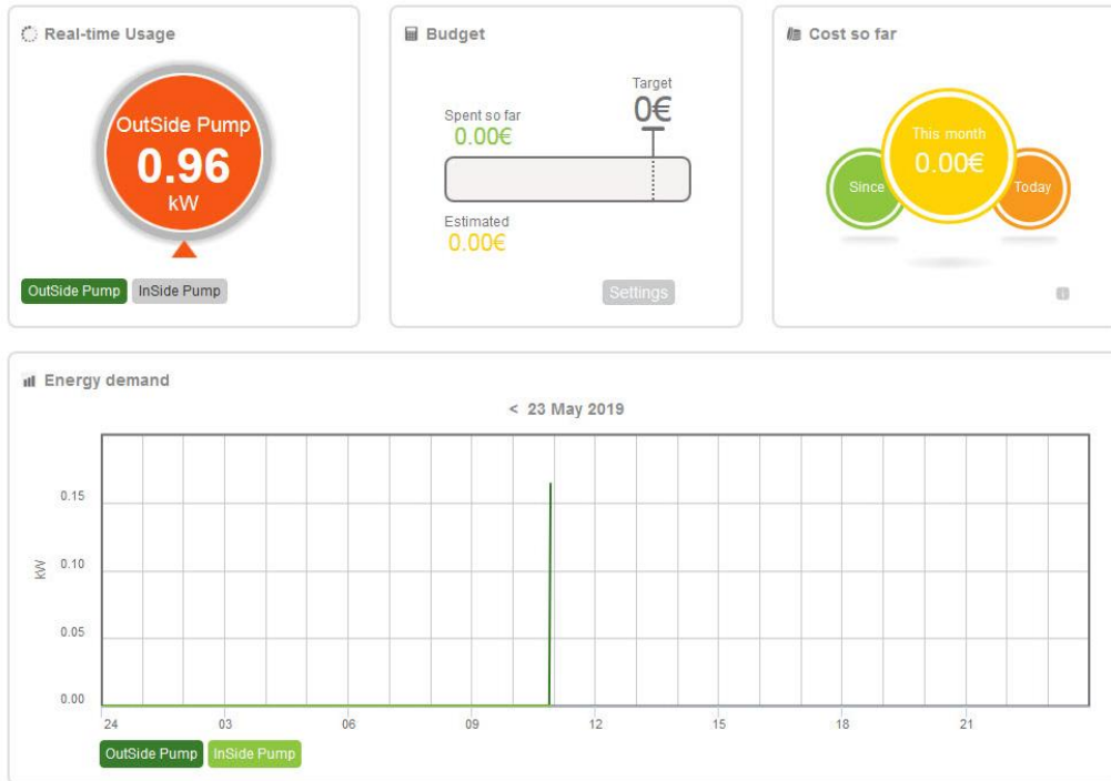
Figure 16. Indicative image of real time power usage recording of Pump C2 (instant power usage value in kW on the top left of the figure and consumption time history at the depicted diagram).
