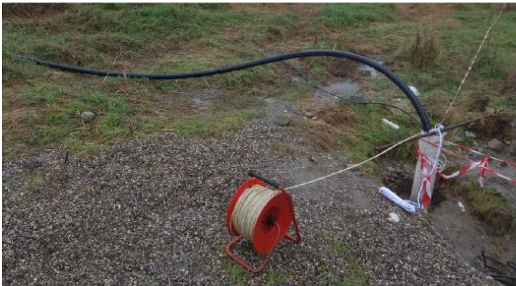
Figure 24. Water pumping during flow testing and simultaneous aquifer depth measurement
