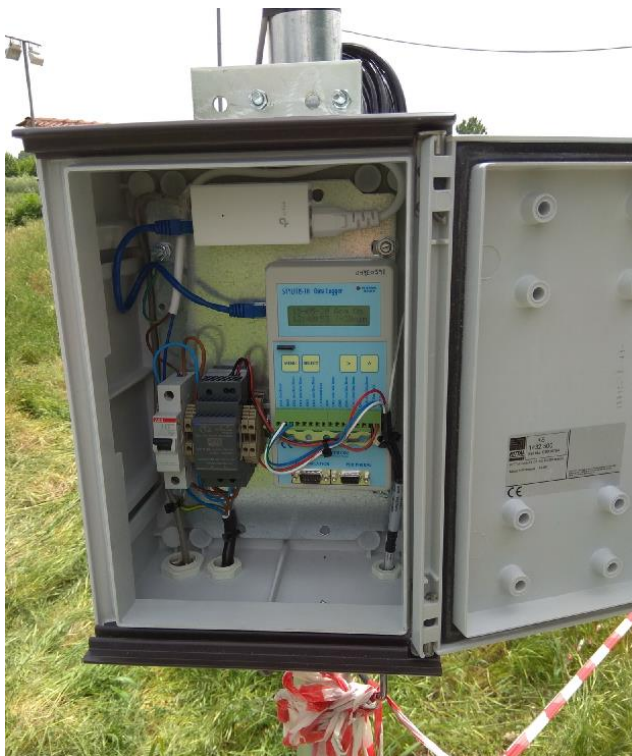
Figure 45. Data logger (left) installed next to the borehole well and submersible sensor (right)
