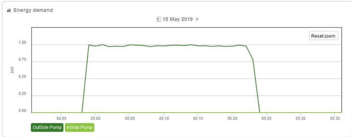
Figure 26. Detail of the recorded usage time history (Pump C2).
